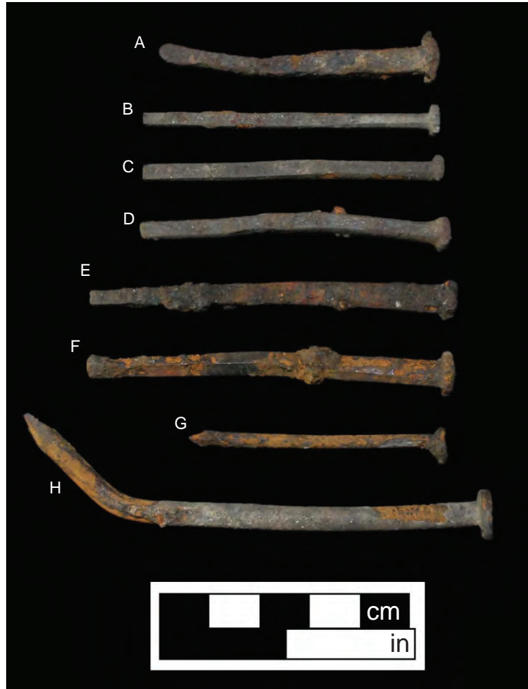
Figure 103. Nails Sub-group A. handwrought nail; B.–F. cut nails; G and H. wire nails
