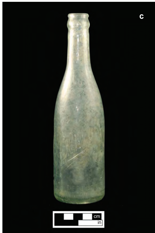
Figure 163. Examples of Glass Bottle Manufacturing Techniques. (a = automatic machine molded; b = blown-in-mold; c = paste or turn molded; d = Ricketts-type molded)
