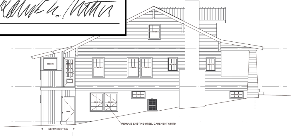
1 D002 EAST ELEVATION - DEMOLITION SCALE: 1/4" = 1'-0"
