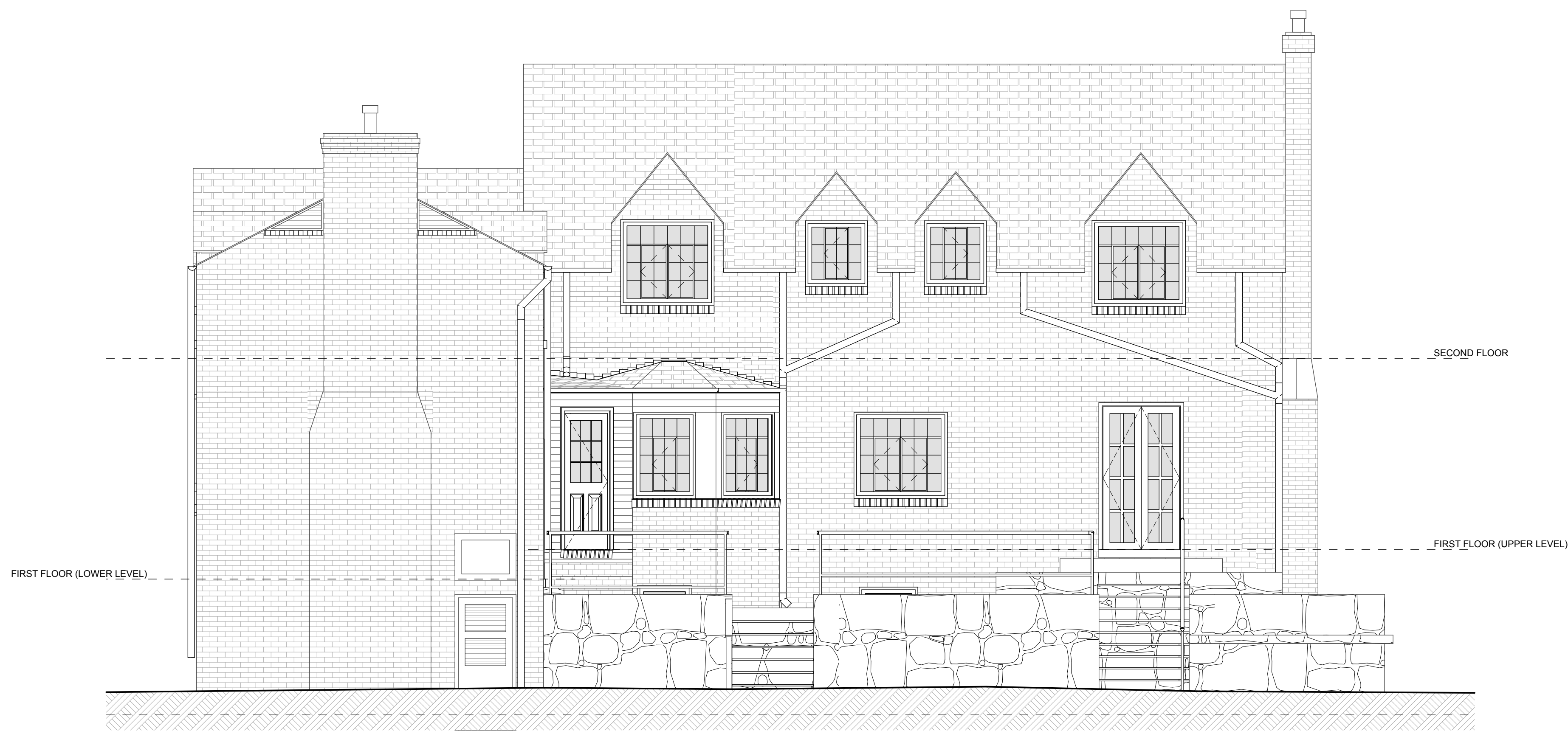
1 A107 EXISTING SOUTHWEST ELEVATION SCALE: 1/4" = 1'-0"
