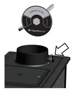
Figure 15 – Catalyst Thermometer
