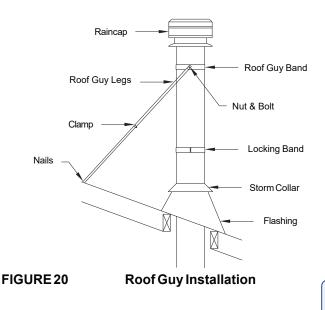
The two telescopic legs should form an angle of about 60 degrees to give support to the chimney in all directions. Keep bottom ends equal distance from the chimney and if possible, at the same elevation, on the high side of the sloped roof. Seal the roof with a suitable non-hardening waterproof caulking. After the legs are attached to the chimney and bands, tighten the clamps on the legs to fix the position of the telescoping legs. (See Figure 20).
