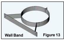
Fasten securely the Wall Band around the chimney with the supplied nut and bolt. Check for clearances and plumb as you fasten the Wall Bands to the wall. Use a level against the chimney section at each support stage to keep the assembly plumb.
