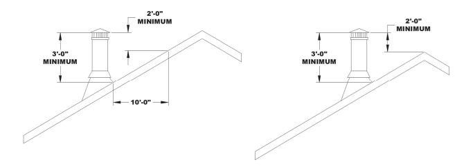
Figure 8 – Chimney Height Requirements
