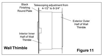
Install the interior inner half (with round plate and tabs) of the wall thimble into the inside wall opening, ensuring that the shield slides over the shield of the exterior outer half (see Figure 11). Once in place and flush against the wall, install the black finishing trim plate (round black plate) onto the inside wall surface and fasten in place with appropriate fasteners through the four pre-punched holes.
