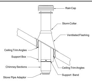
**FIGURE 14 Cathedral Ceiling Support Installation**
