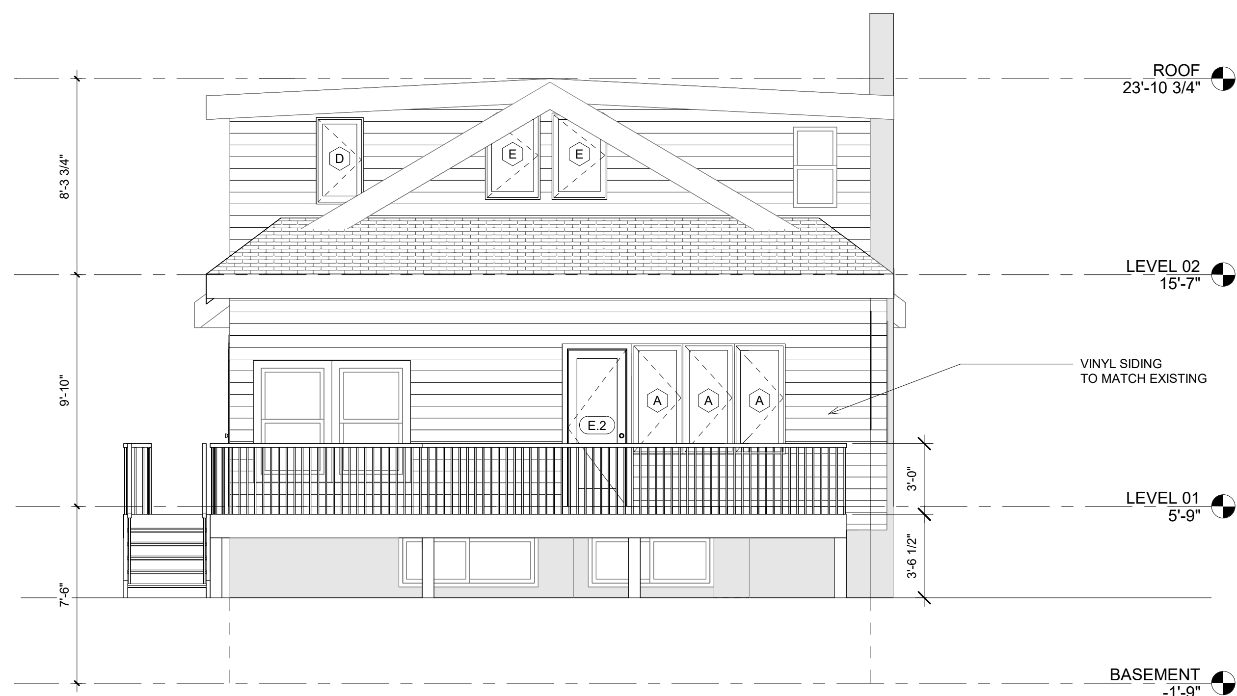
1 WEST ELEVATION - PROPOSED 1/4" = 1'-0" 0' 1 1/2" 3'
