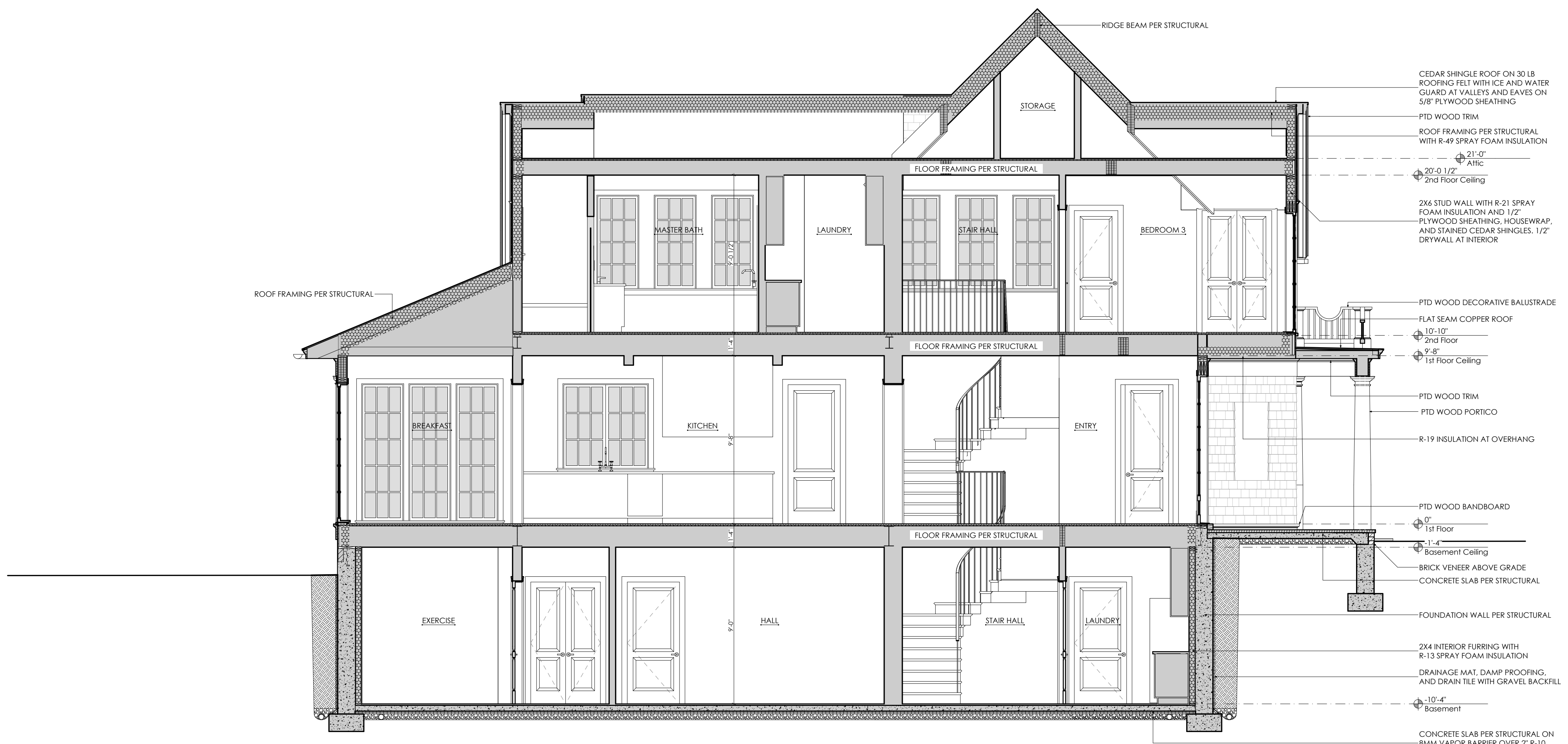
1 Section Through Entry 1/4" = 1'-0"
