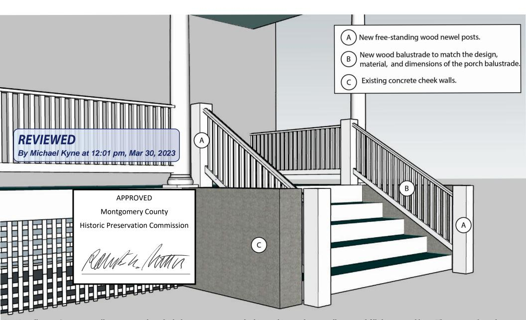
Post Installation: Contractor will cut existing slate, dig hole, pour concrete and rebar, set base anchor, install post, and fill slate around base. The top newel porch will be anchored to the existing porch with a base plate to the existing decking (covered with trim).
