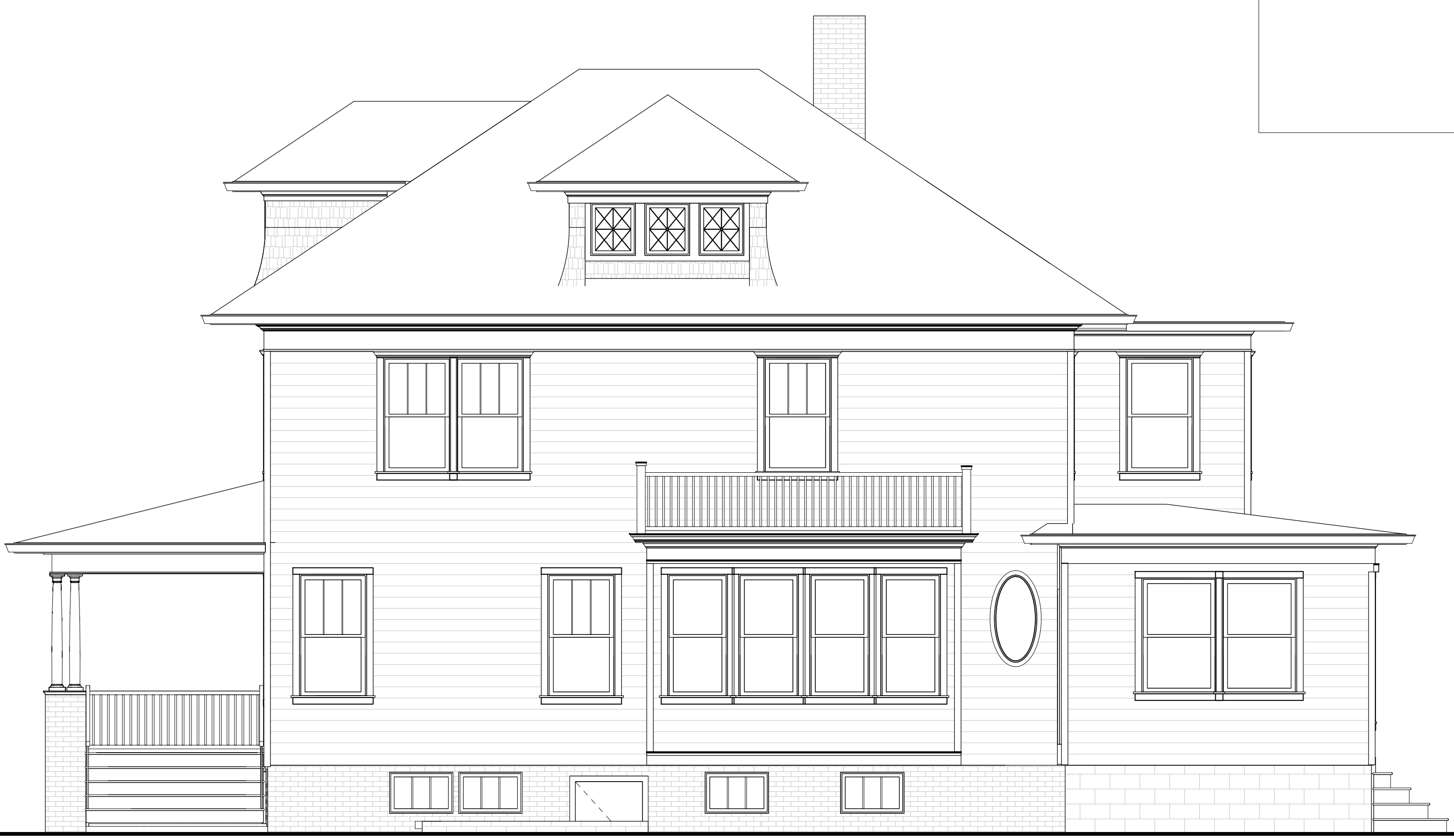
4 Existing Right Elevation 1/4" = 1'-0"
