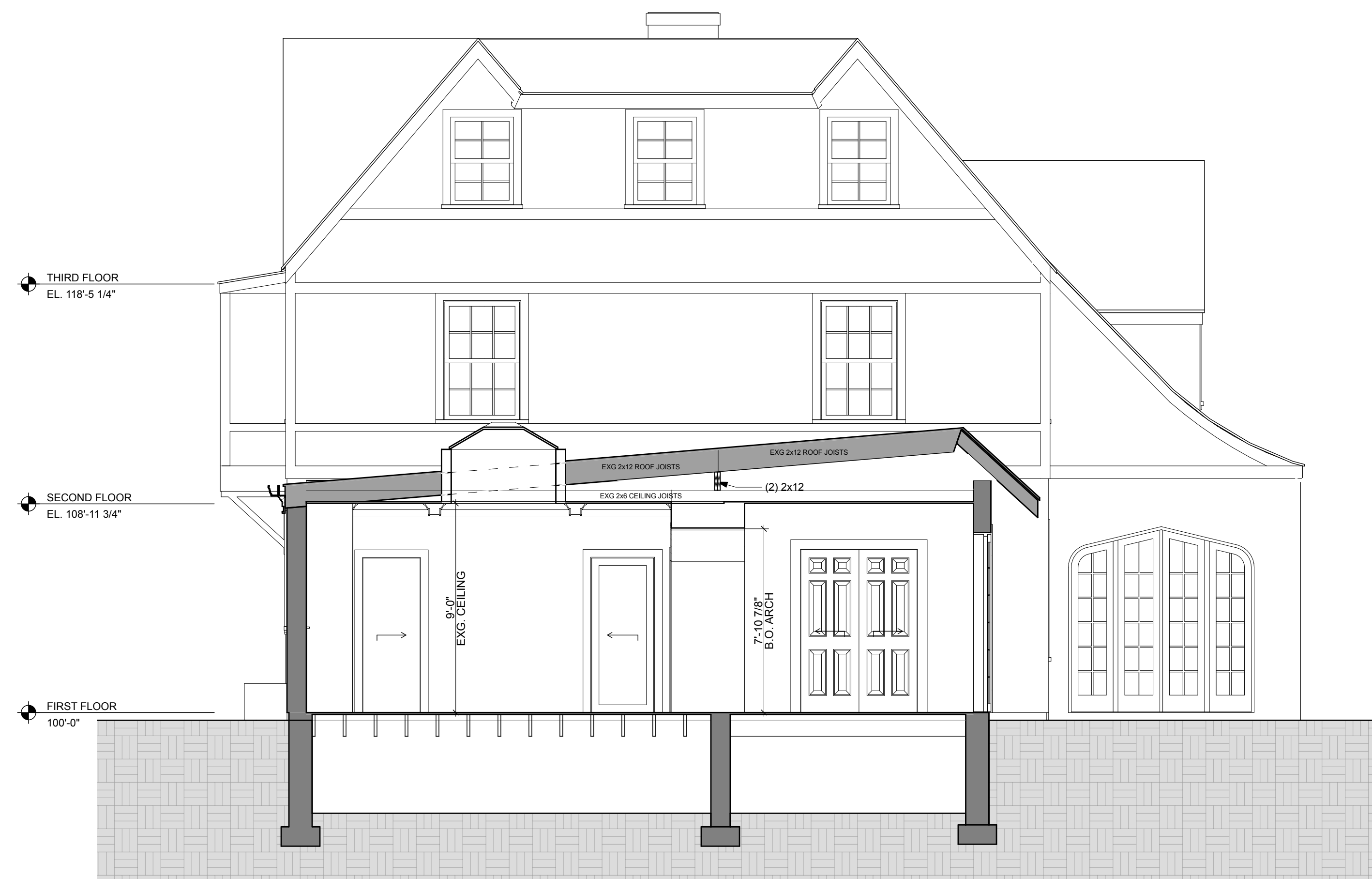
2 SECTION THROUGH KITCHEN SKYLIGHT SCALE: 1/4" = 1'-0"
