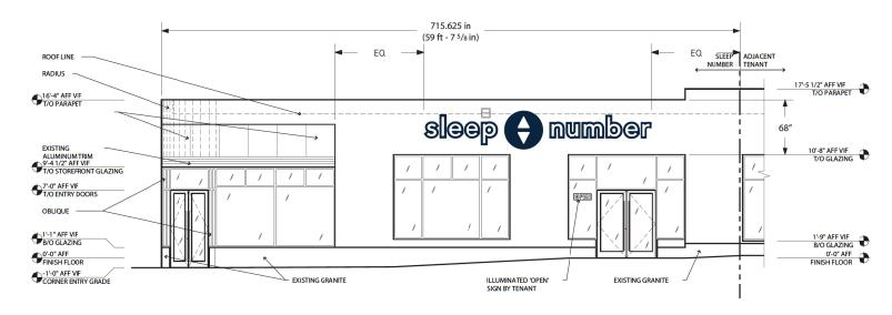
SIGNAGE TO BE PLACED JUST BELOW ROOFLINE (TO CLEAR DRAIN SCUPPER)
