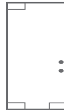
F Style Patch fittings at top and bottom and a lock patch at the leading edge of the door
