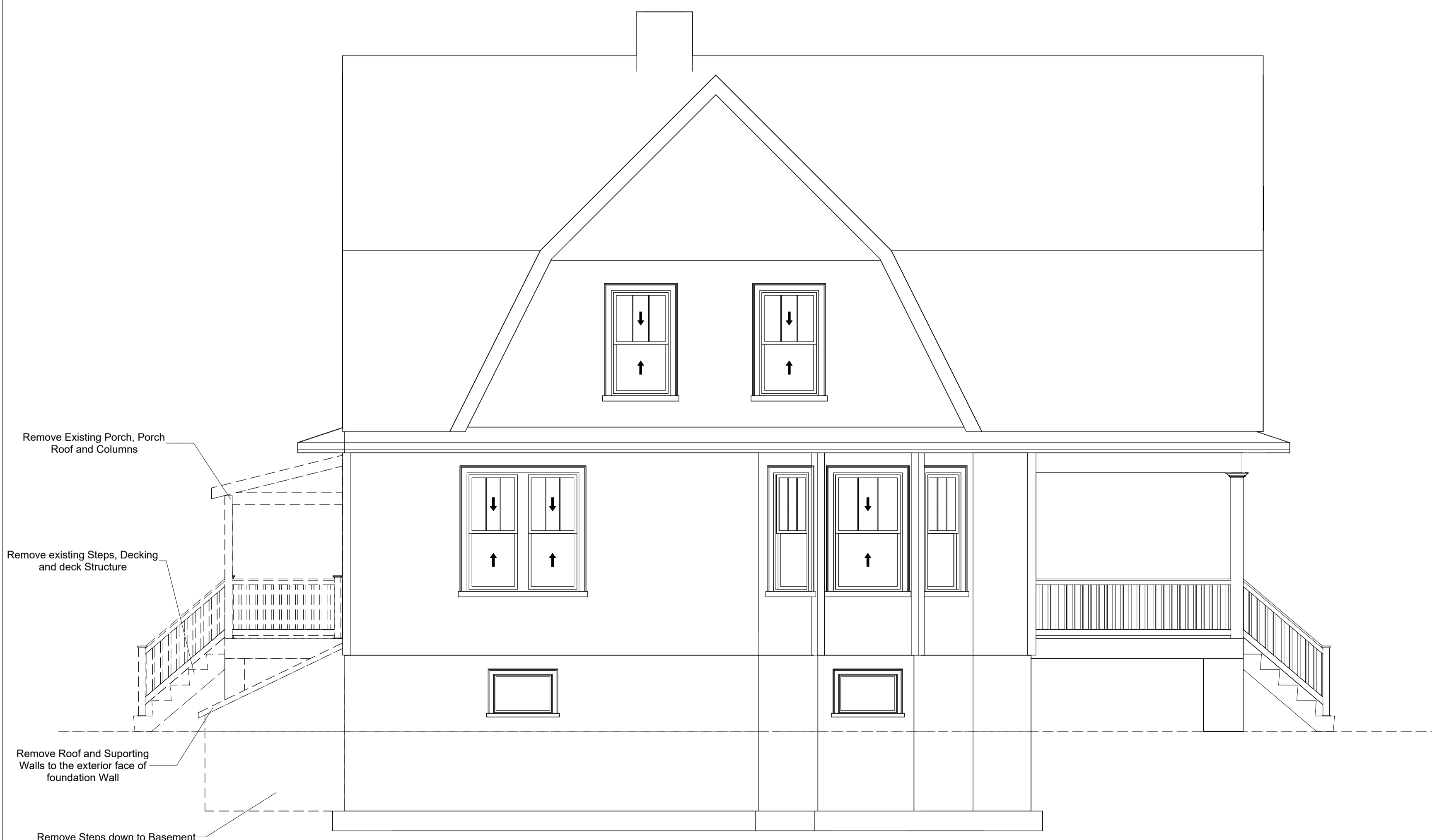
① Right Elevation (Existing) 1/4" = 1'-0"
