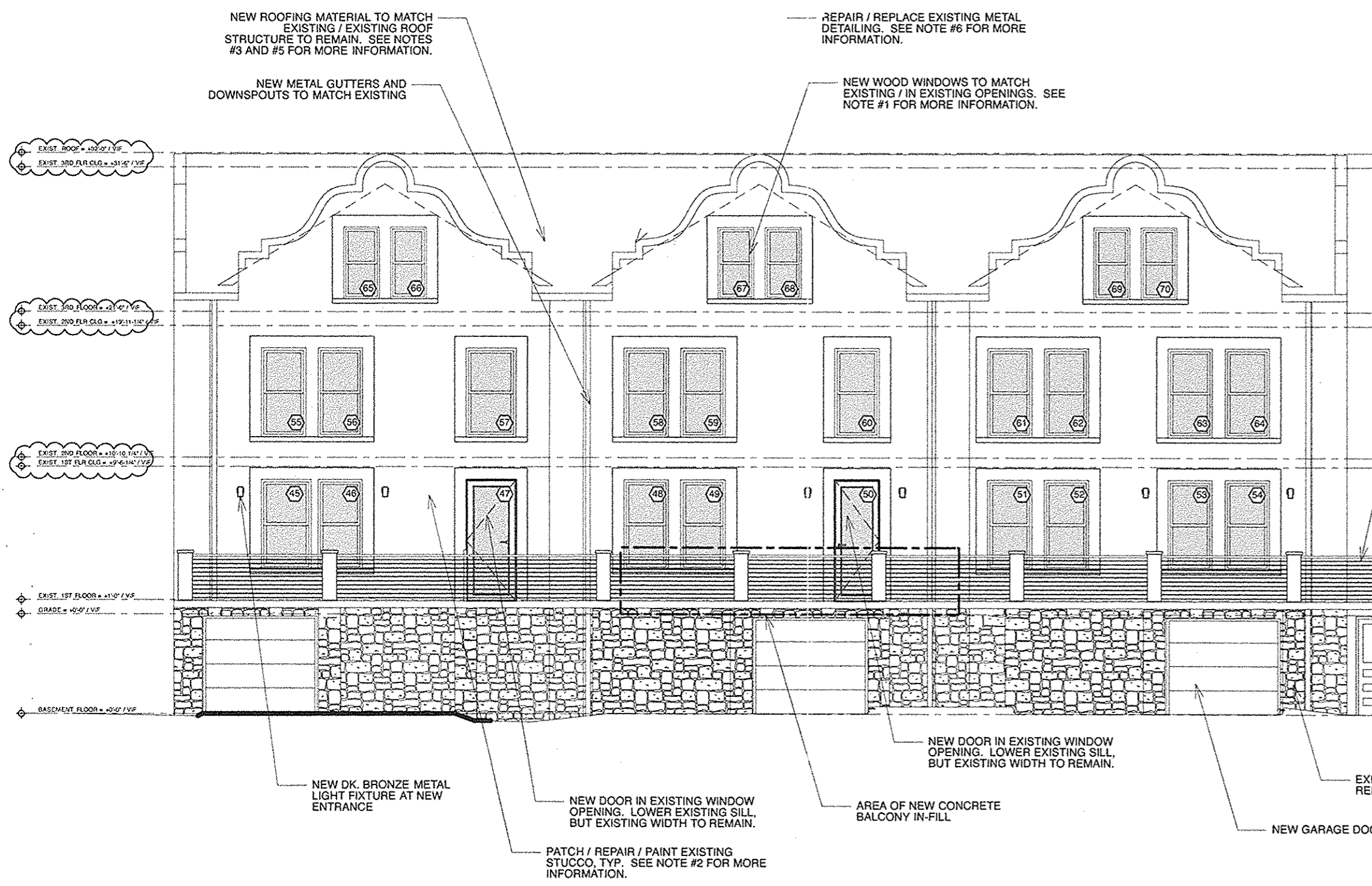
1 NORTH ELEVATION - SERVANT QUARTERS A13 0 1 5 10 20
