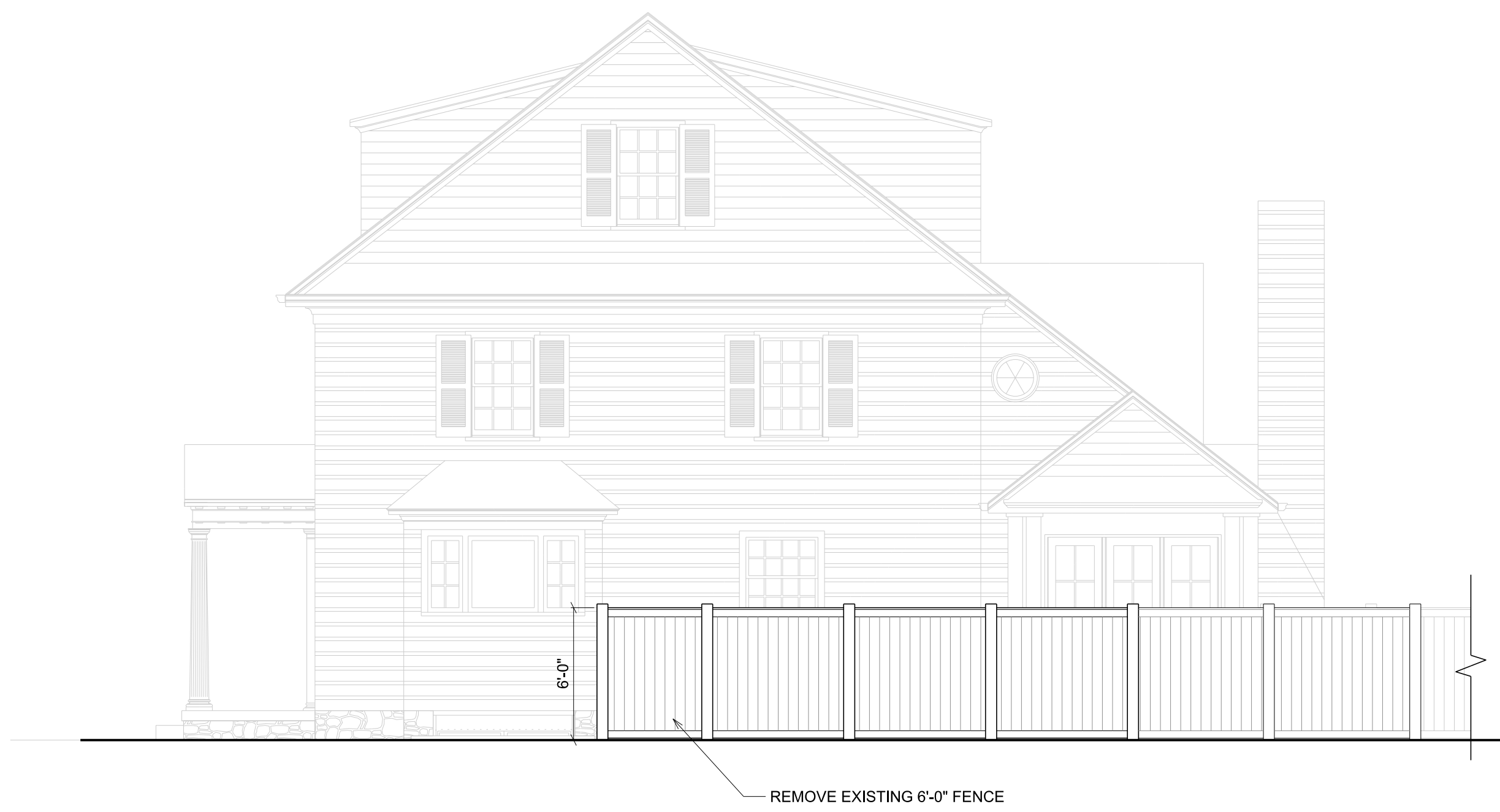
1 EXISTING EAST FENCE ELEVATION A003 SCALE: 3/16" = 1'-0" DEMOLITION
