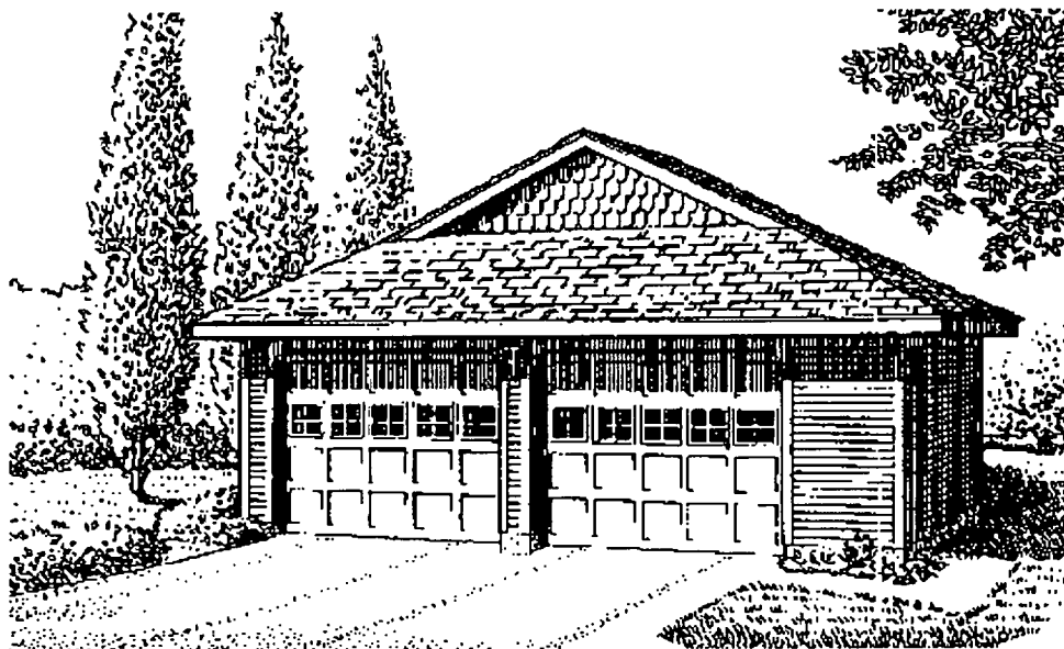
Two-car garage (24' x 24') with clapboard siding and fish-scale shingles.
