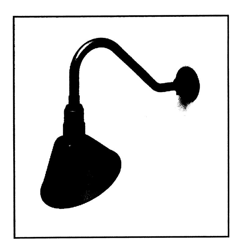
Each outdoor gooseneck light comes with a 4 5/8" diameter round aluminum wall mount back plate and a medium base incandescent ceramic socket wired for 120V service. All back plates have mounting holes that are 3-1/2" on center to allow installation over any standard 4" diameter outdoor recessed (flush mounted) round or octagonal Junction box.
