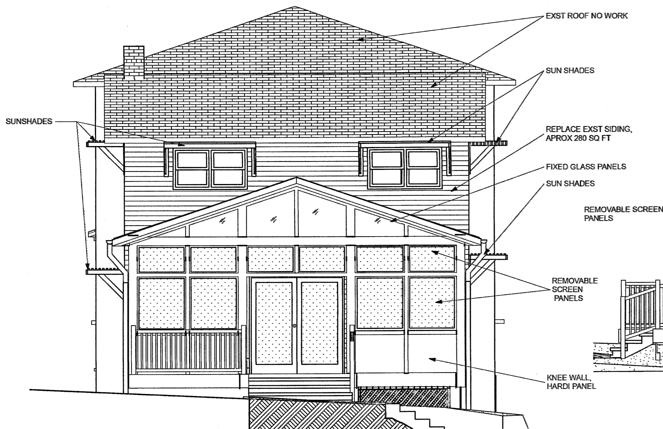
2 North Elevation SCALE: 1/4" = 1'-0"
