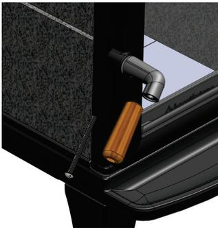
9. Install the catalyst temperature indicator.
