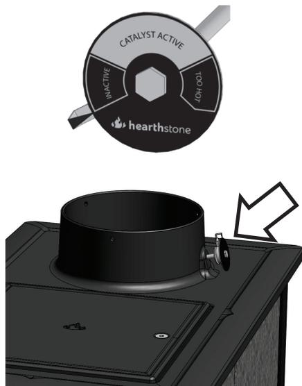
Figure 15 – Catalyst Thermometer
