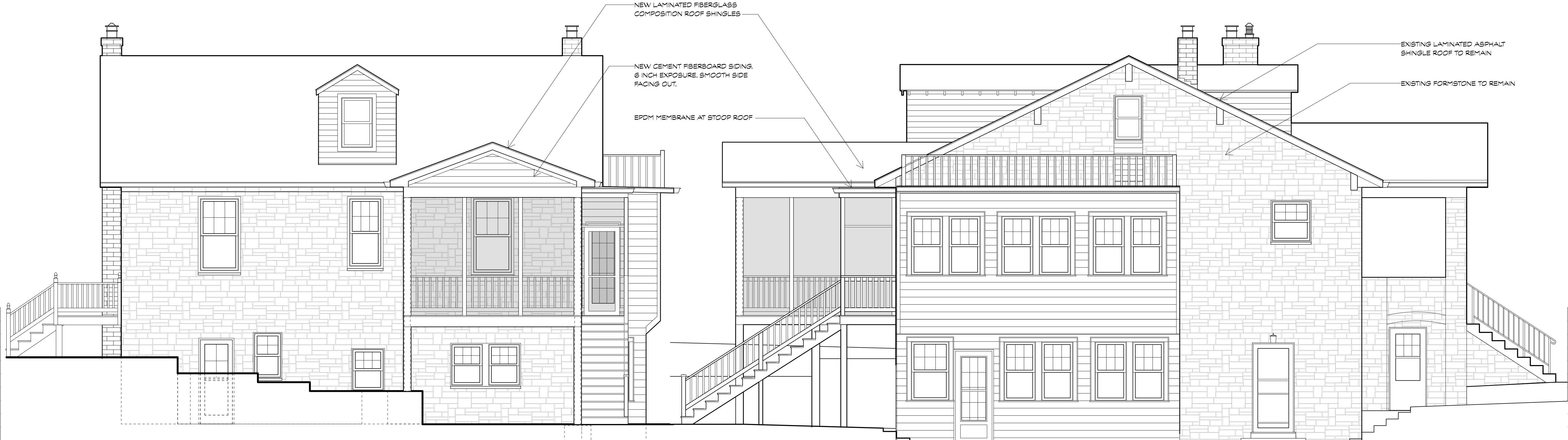
3 PROPOSED REAR ELEVATION Scale: 1/4" = 1'-0"
