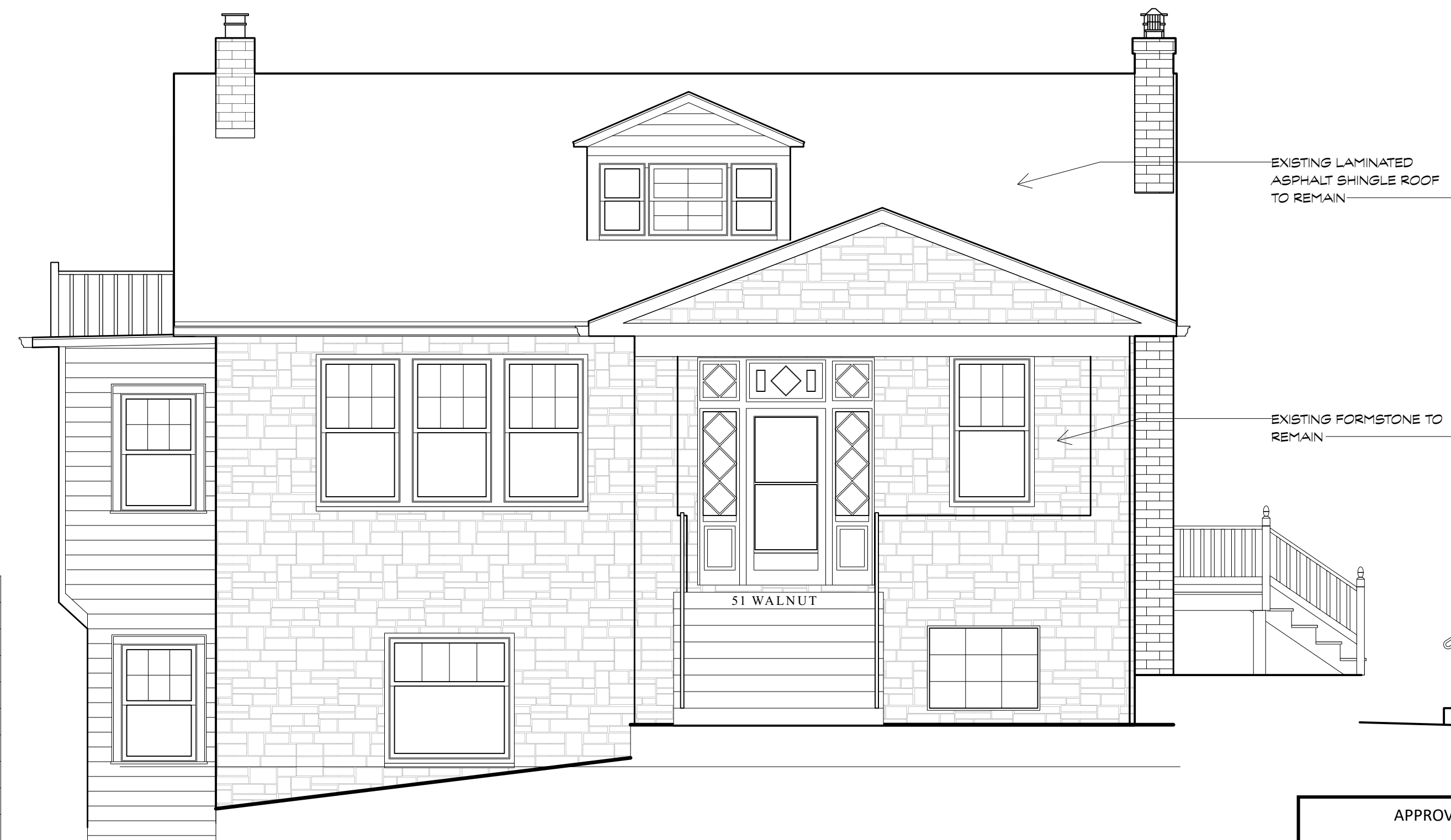
3 PROPOSED FRONT ELEVATION Scale: 1/4" = 1'-0"
