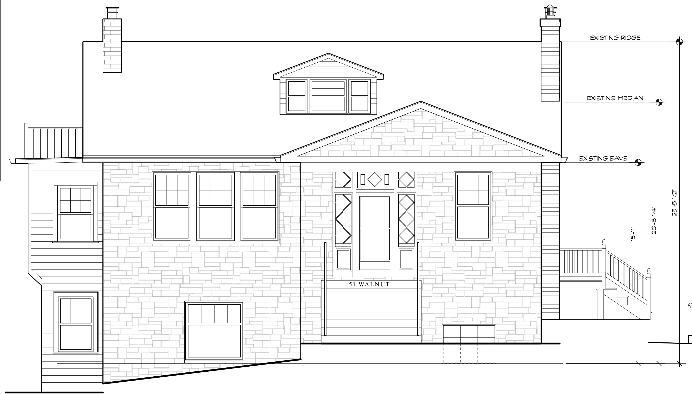
1 EXISTING FRONT ELEVATION Scale: 1/4" = 1'-0"
