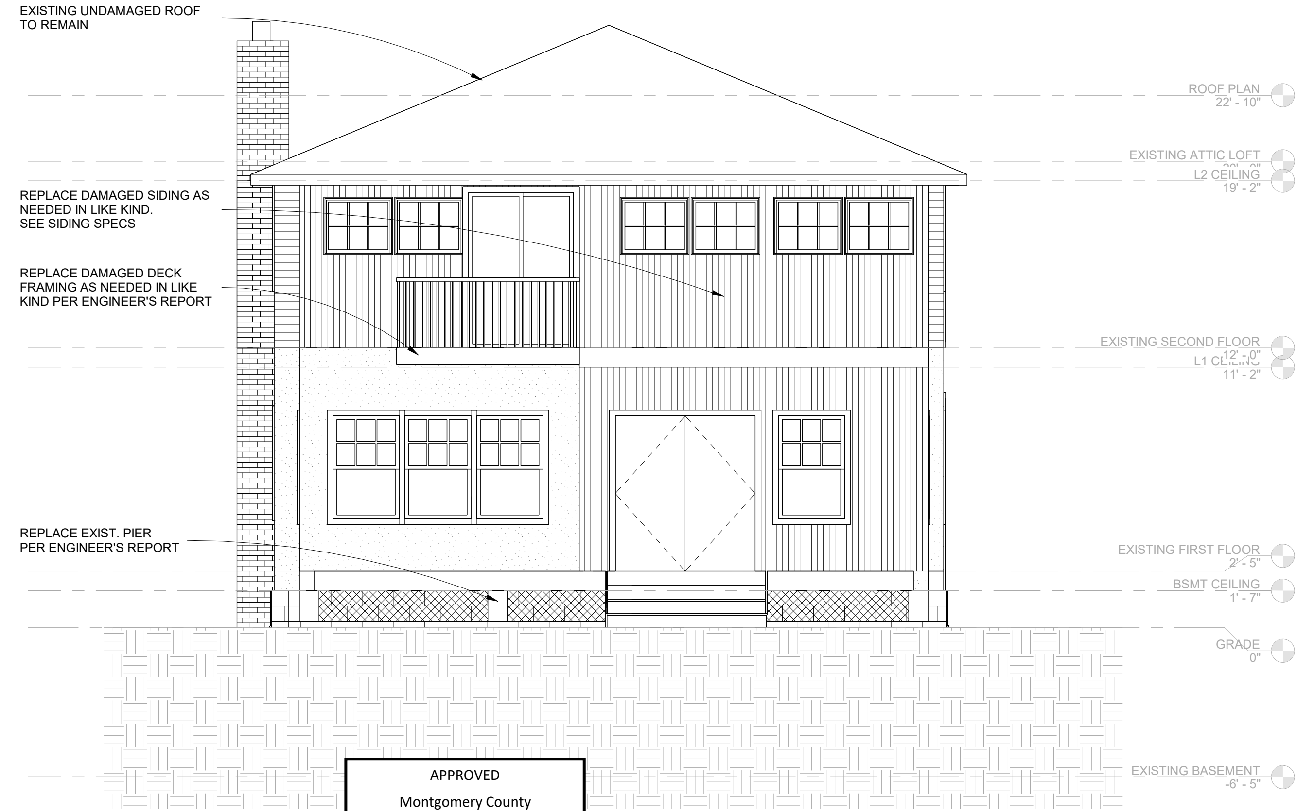
2 EXISTING REAR ELEVATION 1/4" = 1'-0"
