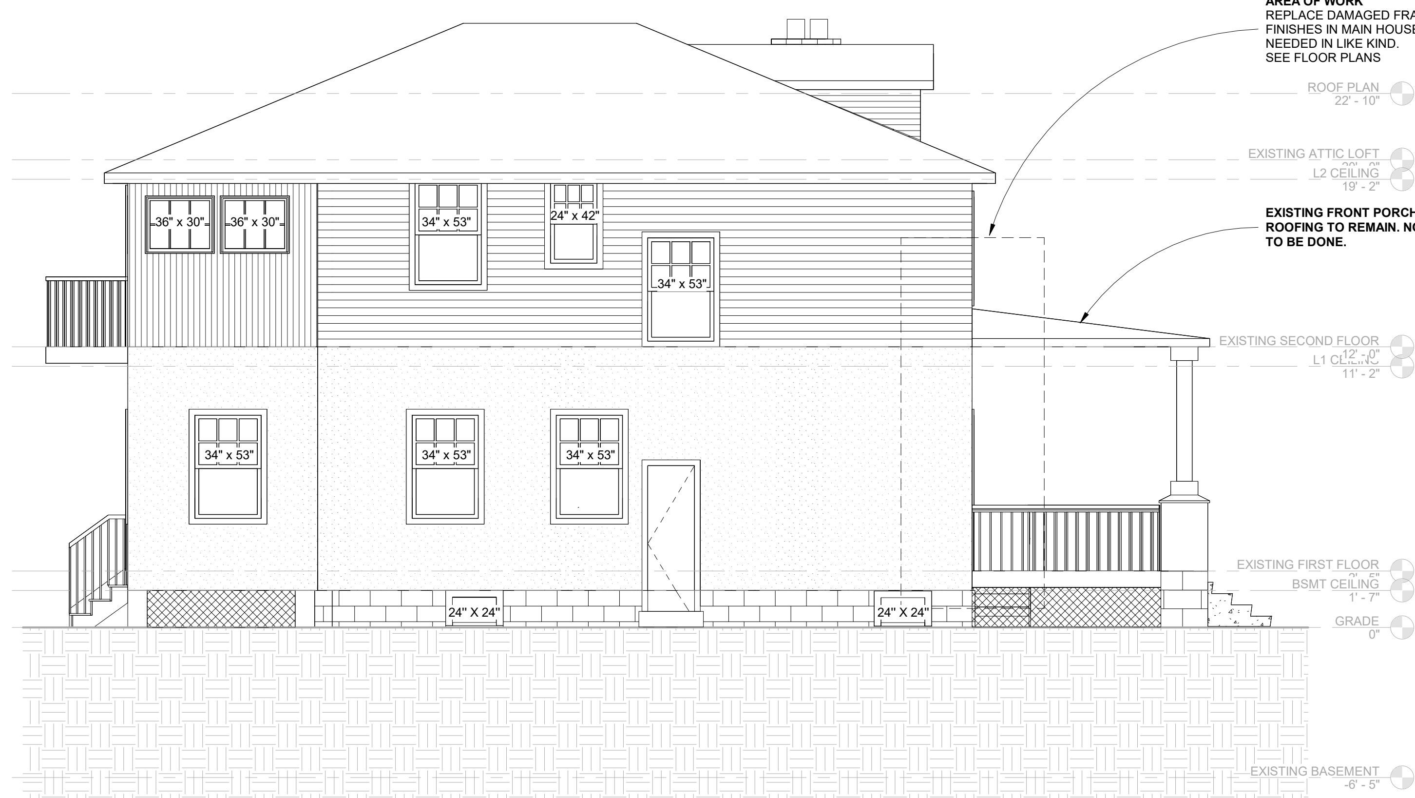
3 EXISTING LEFT ELEVATION 1/4" = 1'-0"
