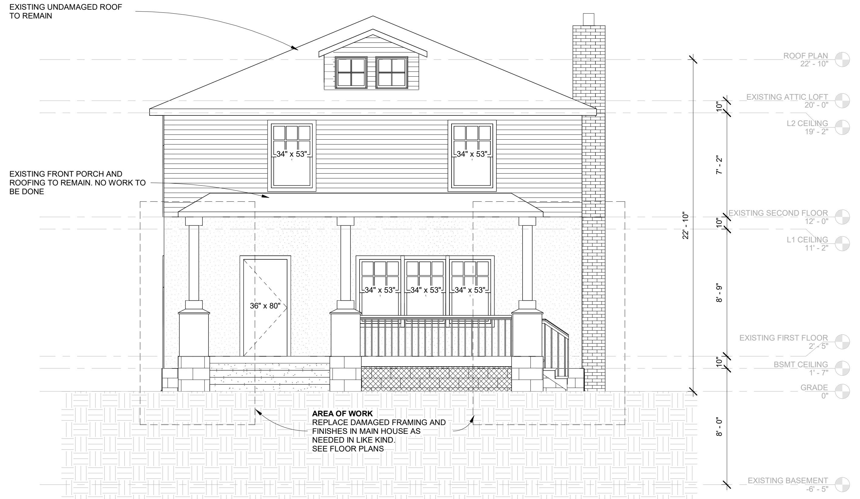
1 EXISTING FRONT ELEVATION 1/4" = 1'-0"
