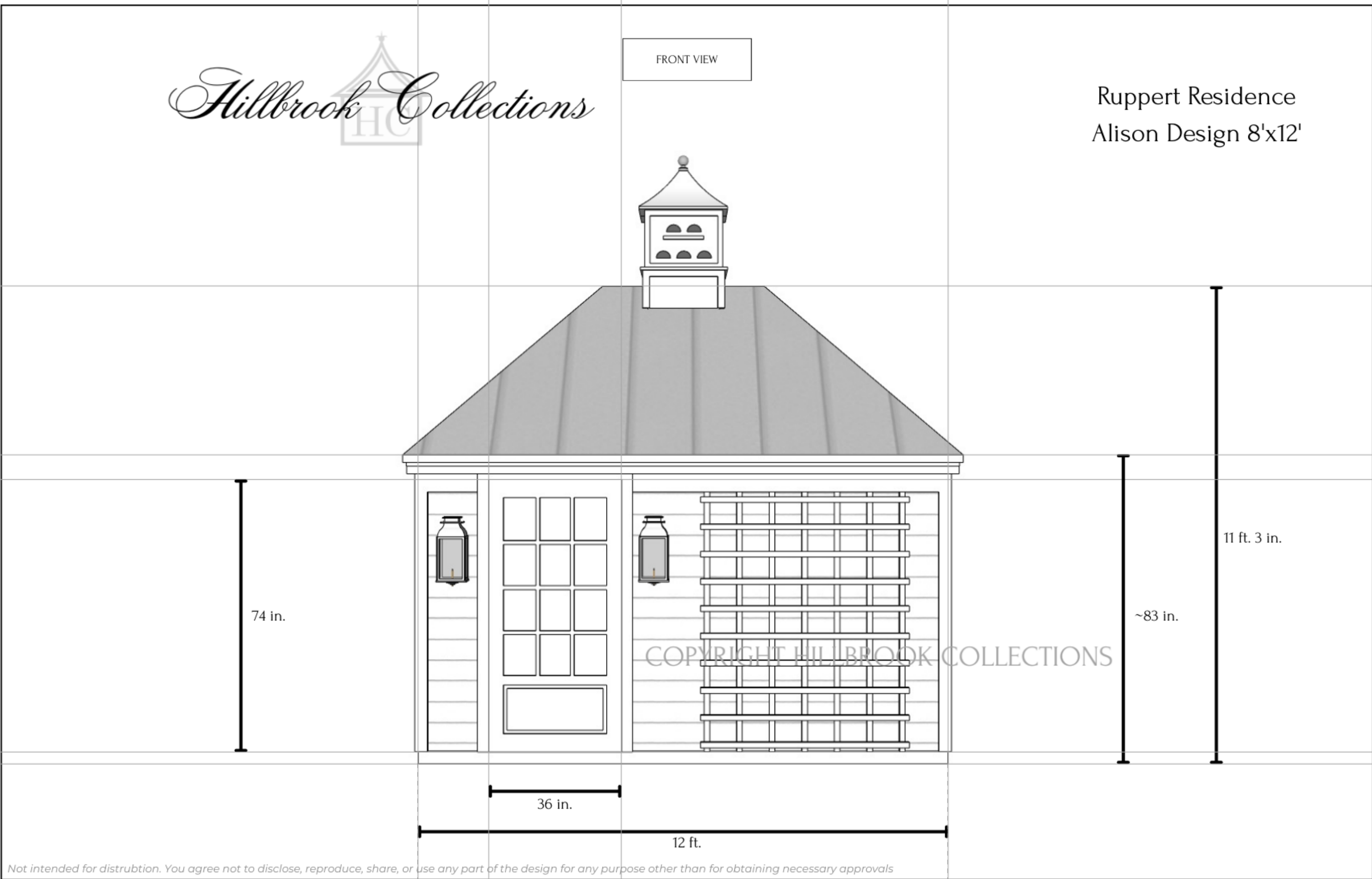
1 Shed Front Elevation 1/2" = 1'-0"
