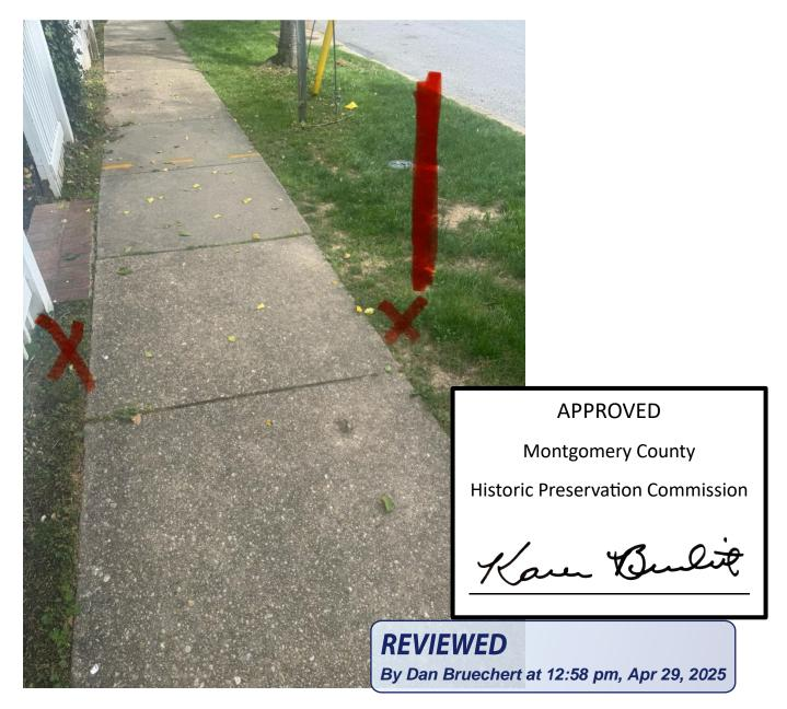
Sample explanation of scope of work: The master electrician will dig from our fence to put in a 2" rigid pipe and dig at the other side of the sidewalk to get to the other end of the pipe. The pipe will be used as a sleeve to run the 1" conduit to power the charger. The charger would be secured on a post facing Baltimore Street in a placement amenable to the city and county.
