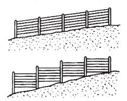
On gentle slopes, the fence follows the slope. On steep slopes, the fence is stepped accordingly.
