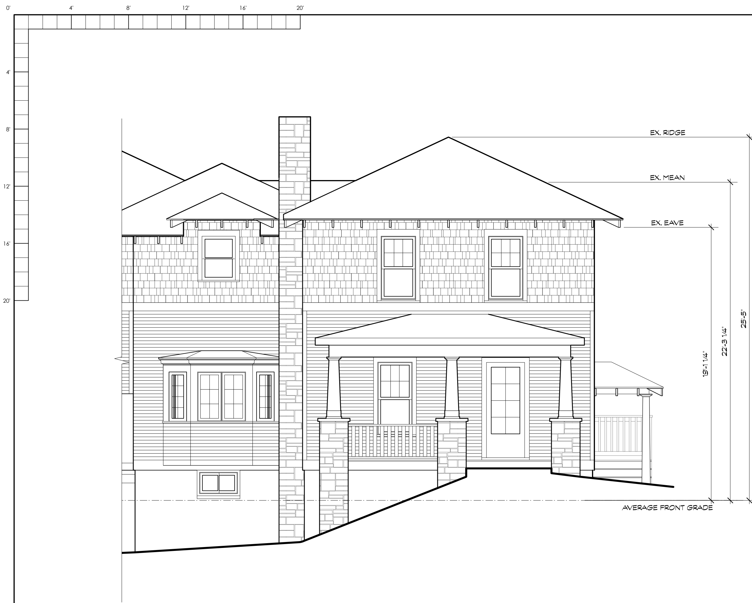
1 EXISTING FRONT (WEST) ELEVATION Scale: 1/4" = 1'-0"
