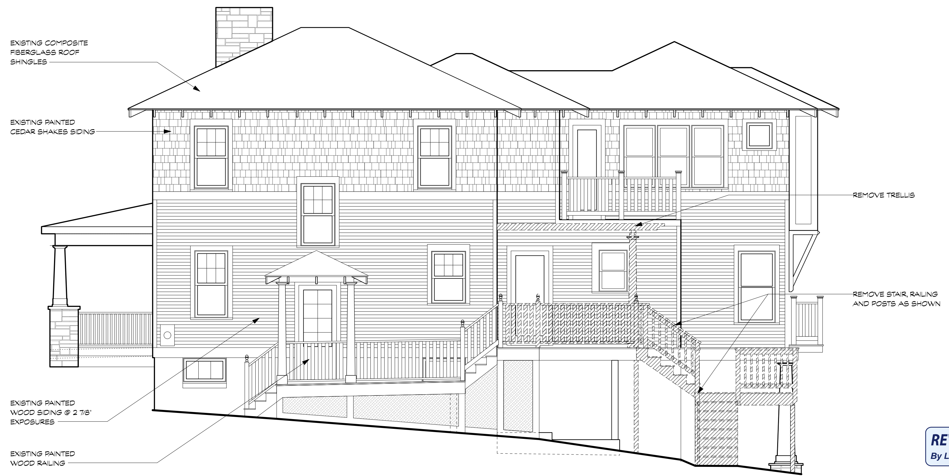
2 DEMOLITION SIDE (SOUTH) ELEVATION Scale: 1/4" = 1'-0"
