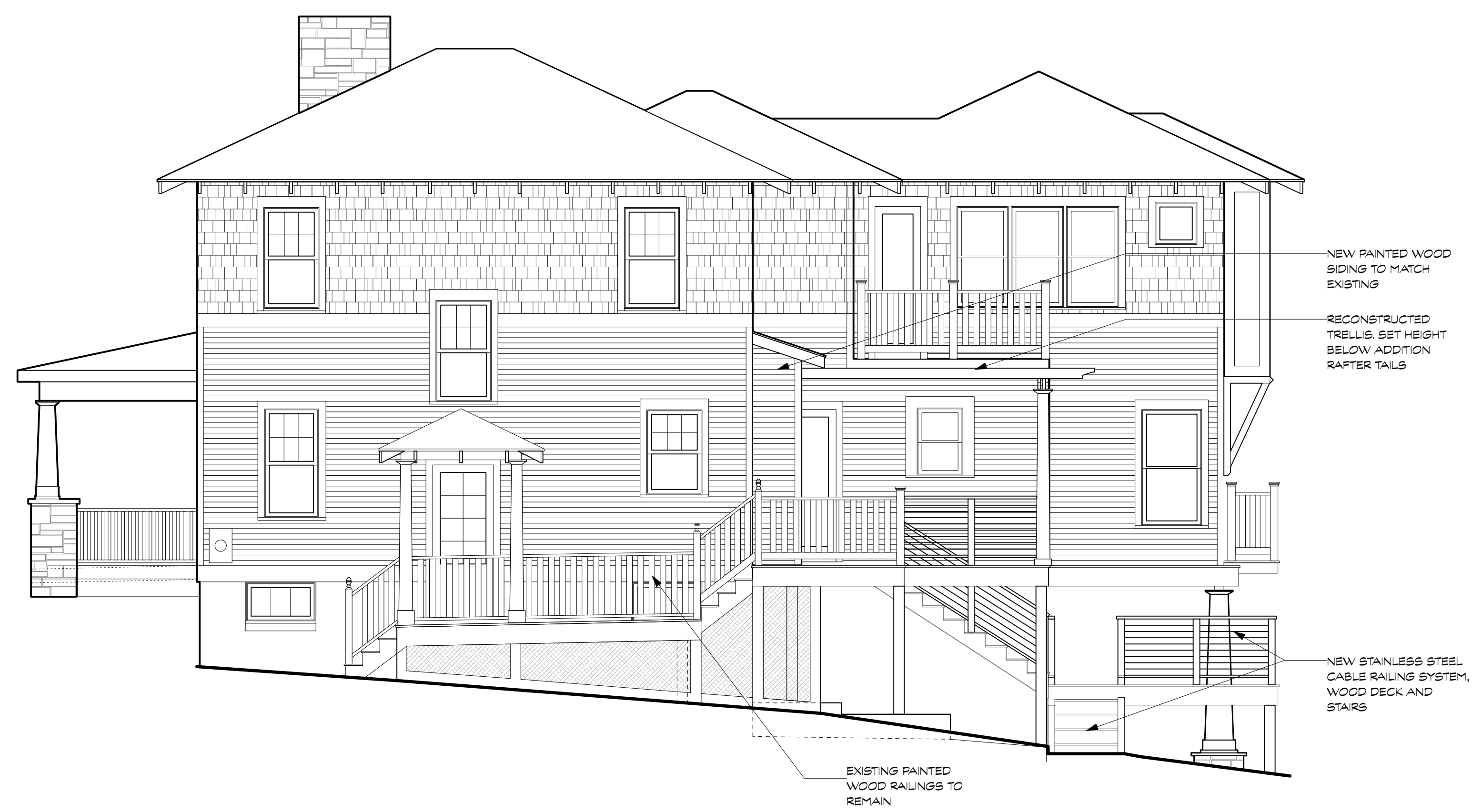
3 PROPOSED SIDE (SOUTH) ELEVATION Scale: 1/4" = 1'-0"
