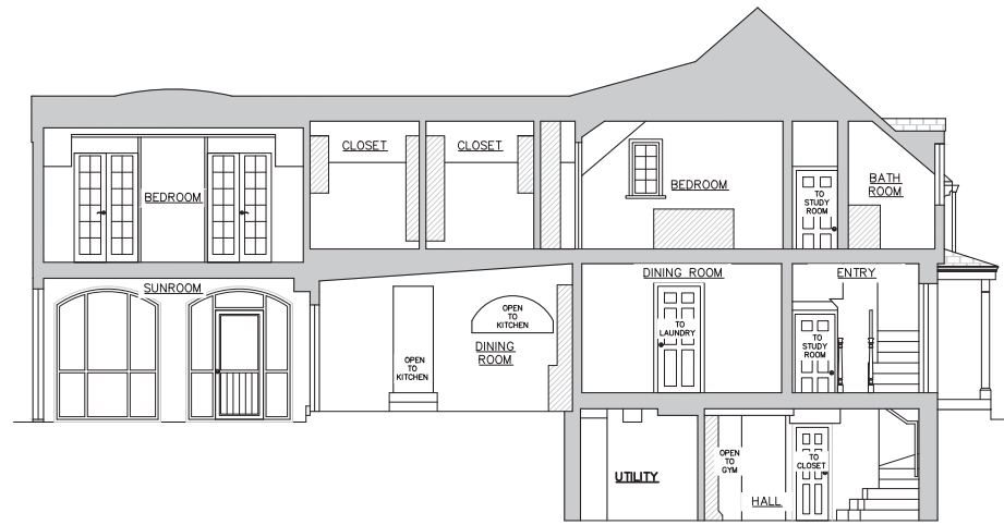
1 A-502 EXISTING BUILDING SECTION SCALE: 1/4" = 1'-0"
