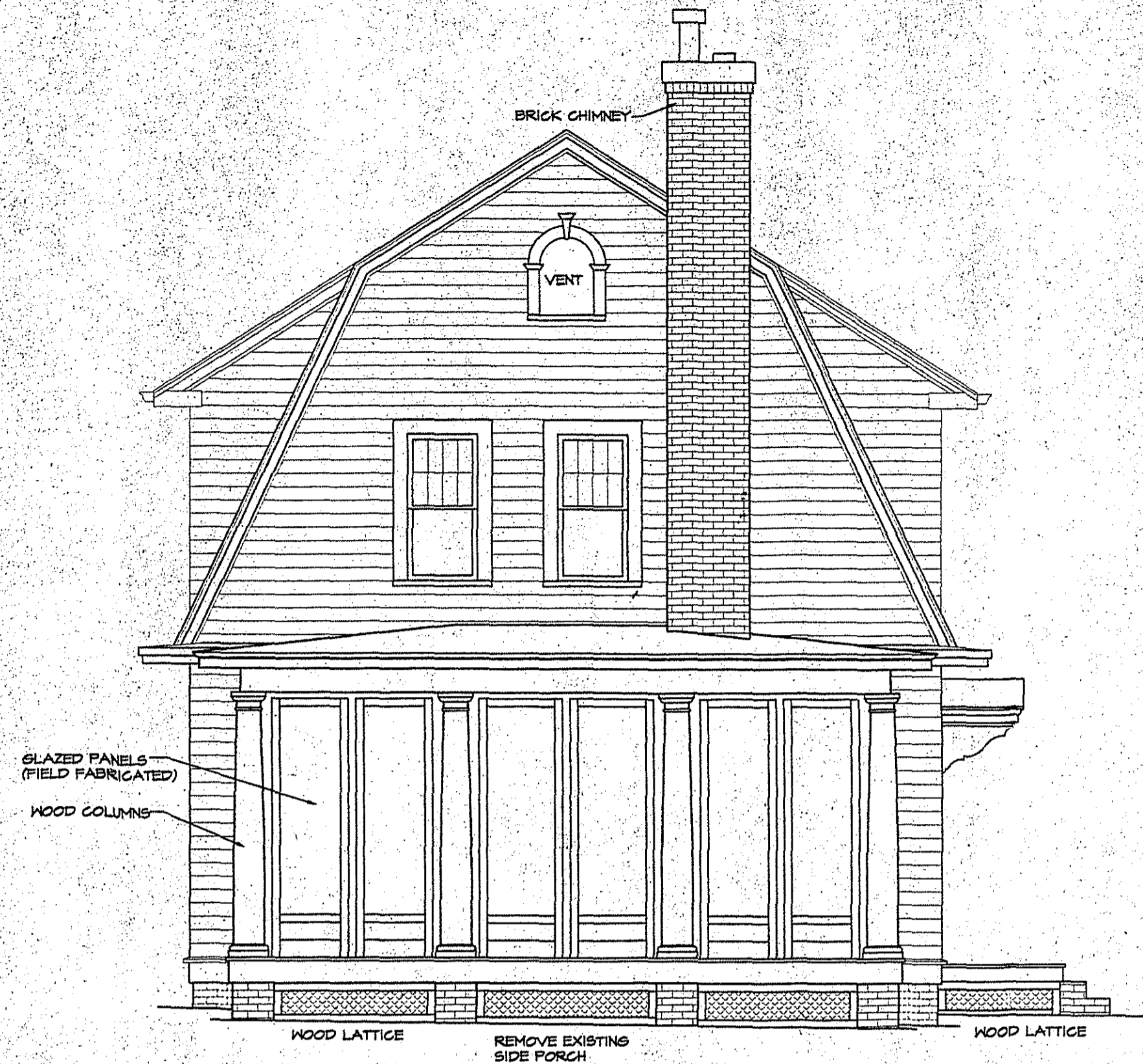
EXISTING NORTHEAST ELEVATION SCALE 1/4"=1'-0"
