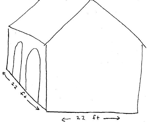
we would like to keep the arches on the north side by making them windows with paned glass. Add skylights on either side
