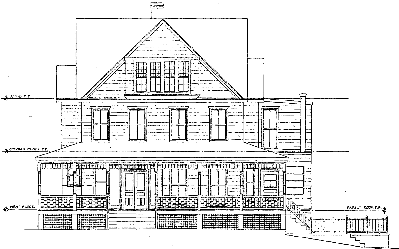
SOUTH ELEVATION, EXISTING SCALE : 1/8" = 1'-0"
