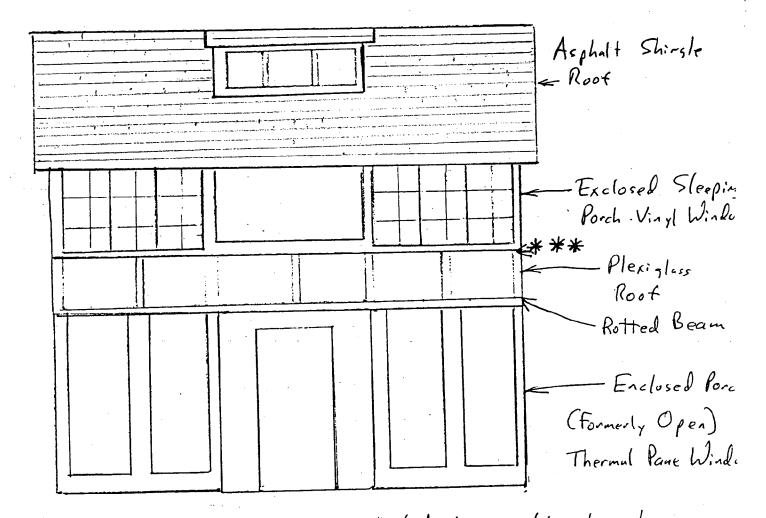
\*\*\* Plexiglass roof was attached incorrectly to house allowing water to seep in causing beam to not.
