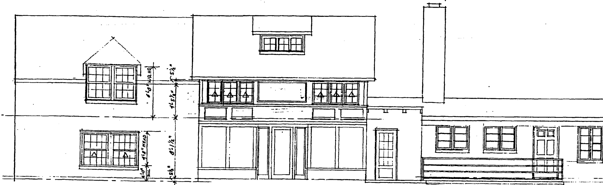
SOUTH ELEVATION (EXIST.) 1/4" = 1'-0"
