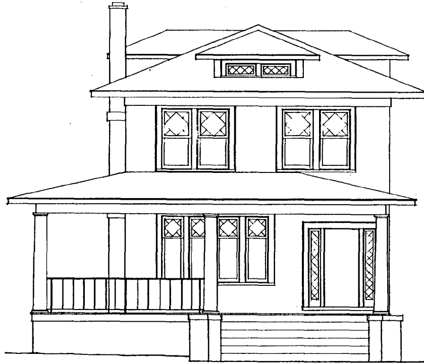
EXISTING EAST ELEVATION 1/4" = 1'-0"
