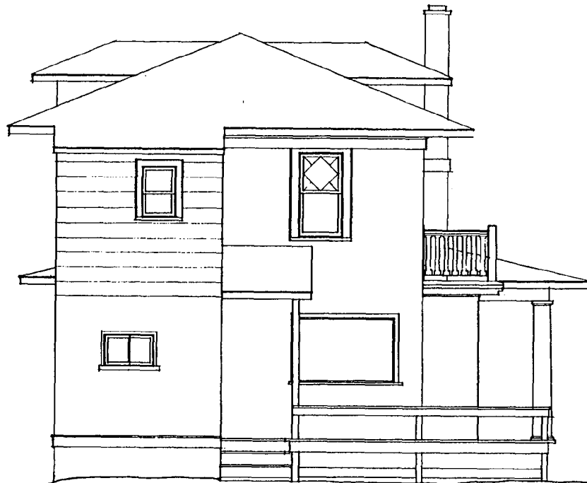
EXISTING WEST ELEVATION 1/4" = 1'-0"
