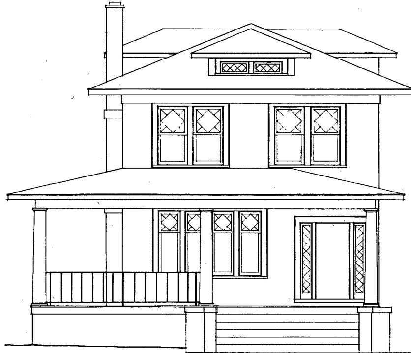
EXISTING EAST ELEVATION 1/4" = 1'-0"
