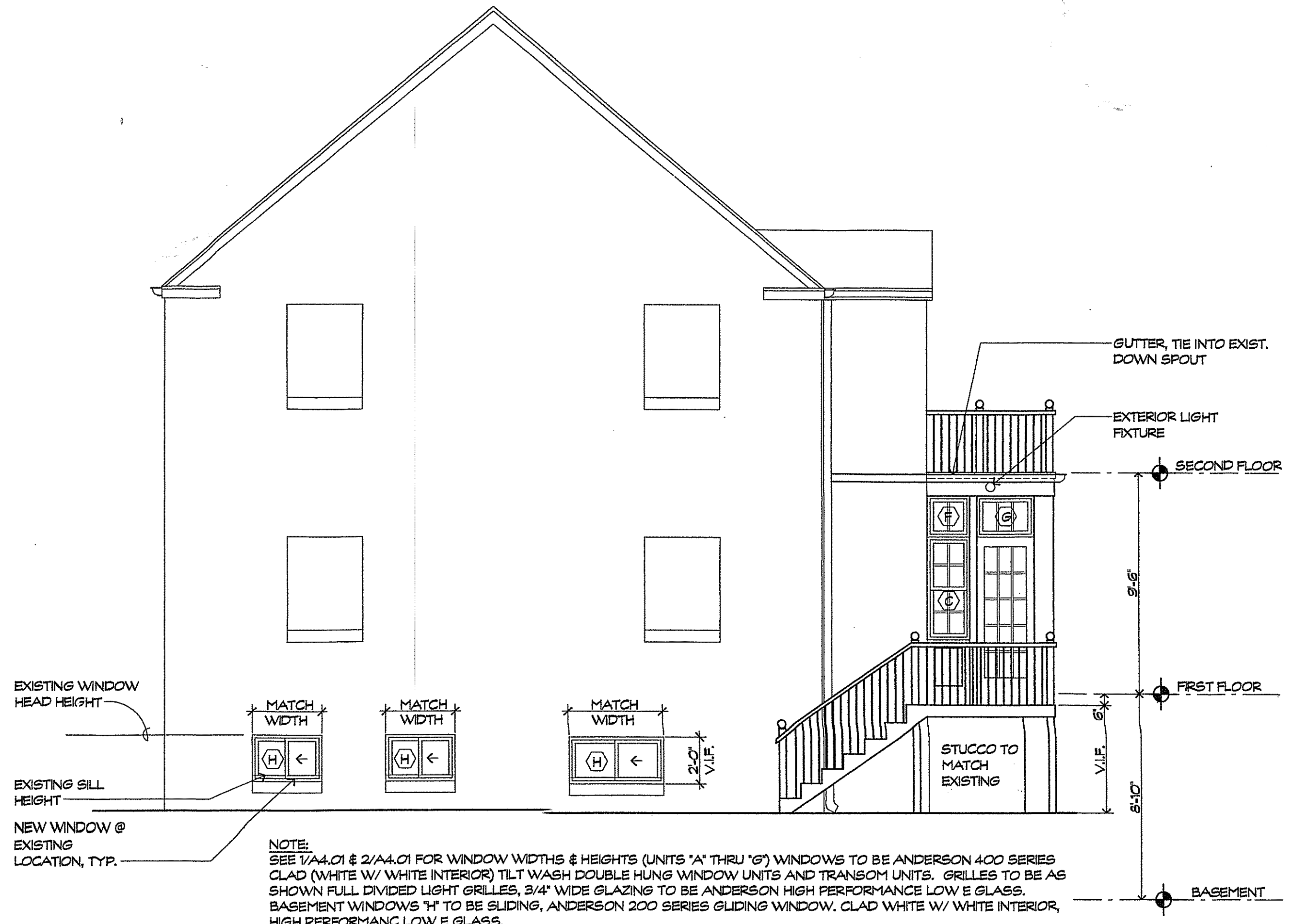
1 ELEVATION EAST SOUTH FACADE A3.01 SCALE 1/4"=1'-0"
