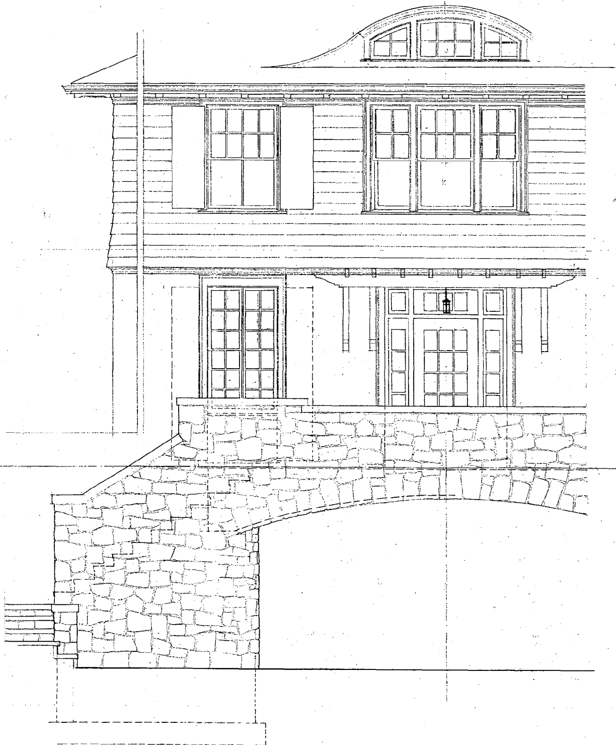
1 A-1 DETAIL ELEVATION @ SOUTH 3/4" = 1'-0"
