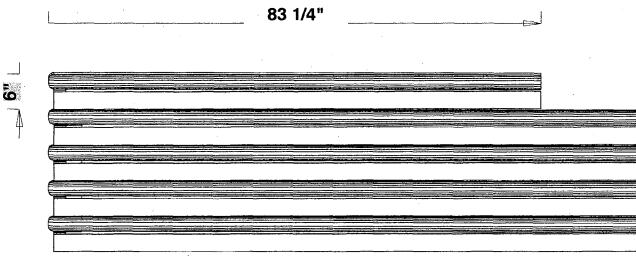
2" Indiana limestone treads & risers w/ 1/4" joints per plan typ. full radius nose
