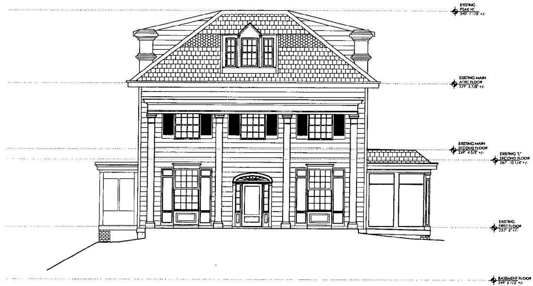
1 EX2.3 EXISTING SOUTH FRONT STREET ELEVATION SCALE: 1/4" = 1'-0"
