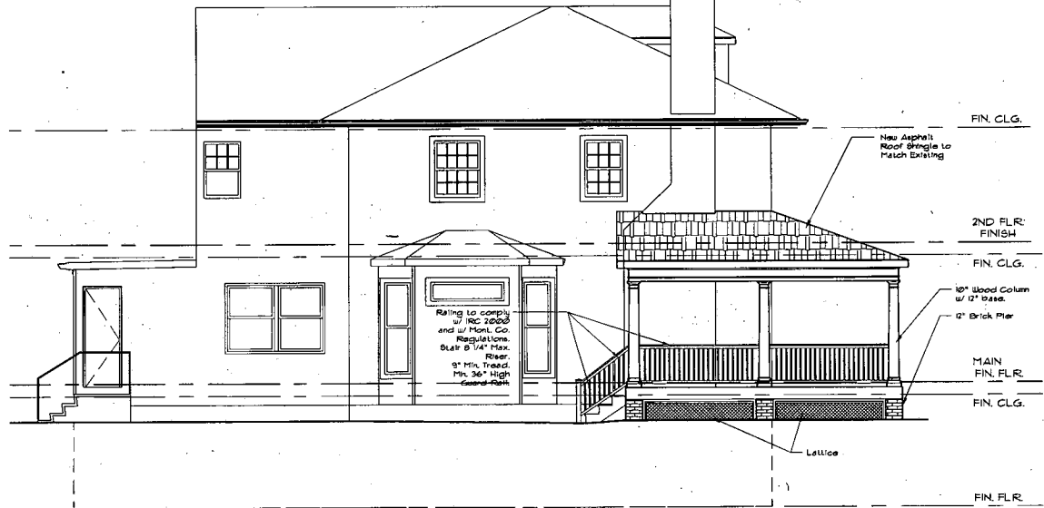
PROPOSED LEFT SIDE ELEVATION SCALE 1/4" = 1'-0"
