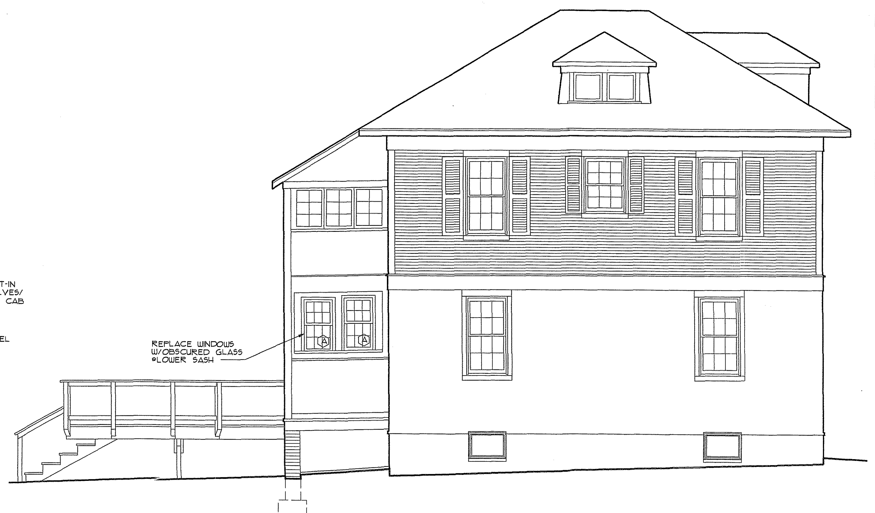
3 PROPOSED NORTHWEST ELEVATION SCALE: 1/4" = 1'-0"
