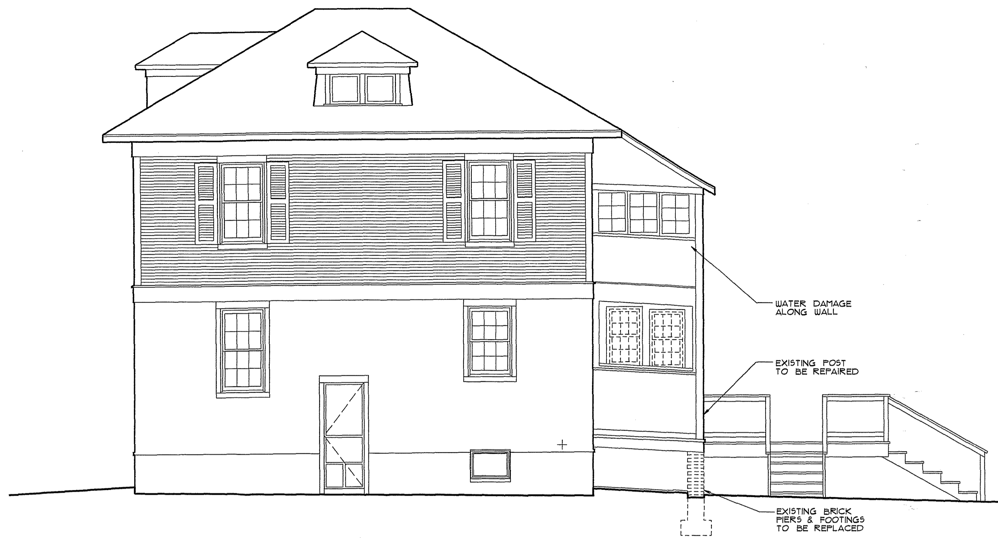
1 DEMOLITION SOUTHEAST ELEVATION SCALE: 1/4" = 1'-0"
