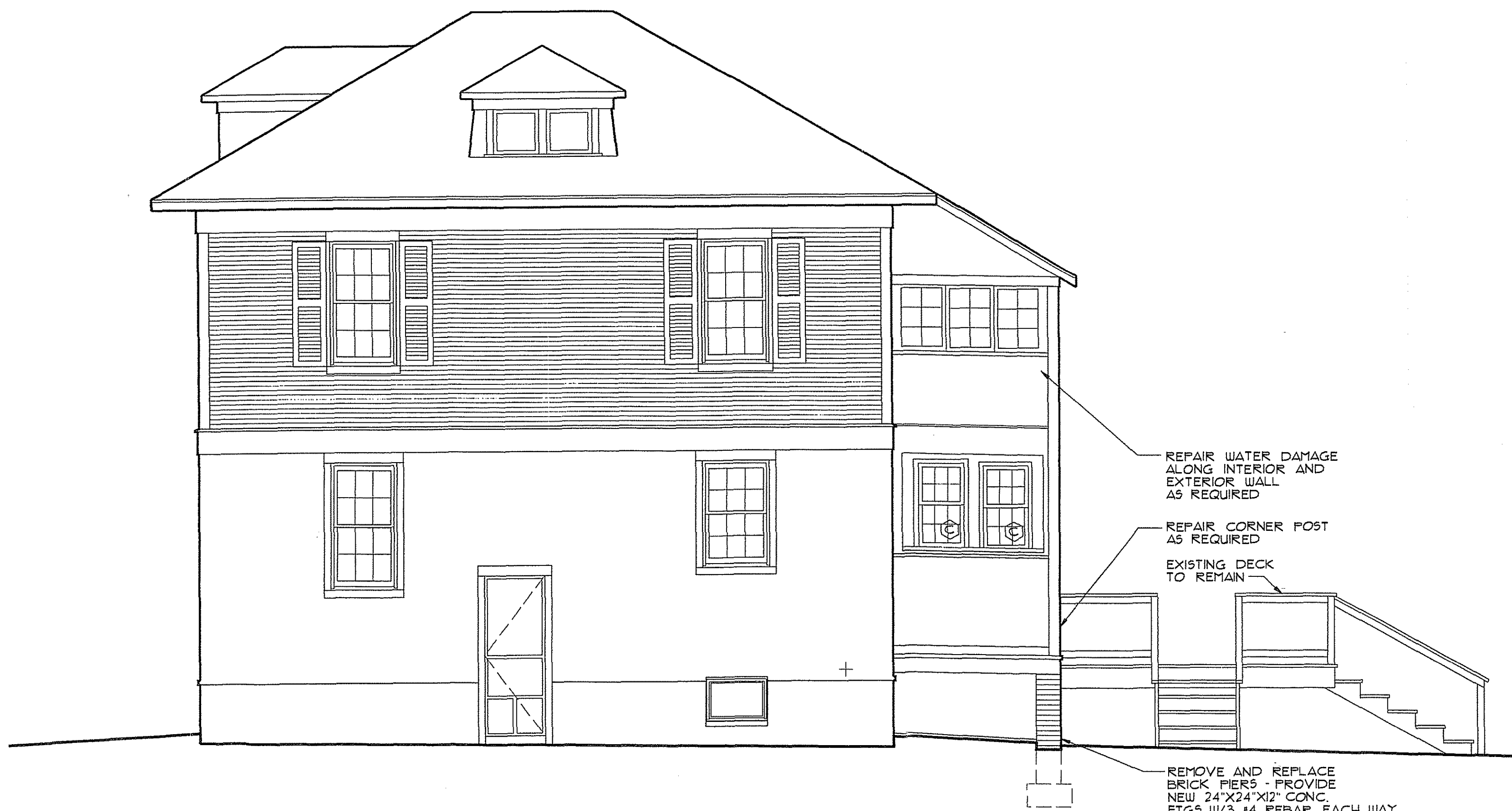
1 PROPOSED SOUTHEAST ELEVATION SCALE: 1/4" = 1'-0"
