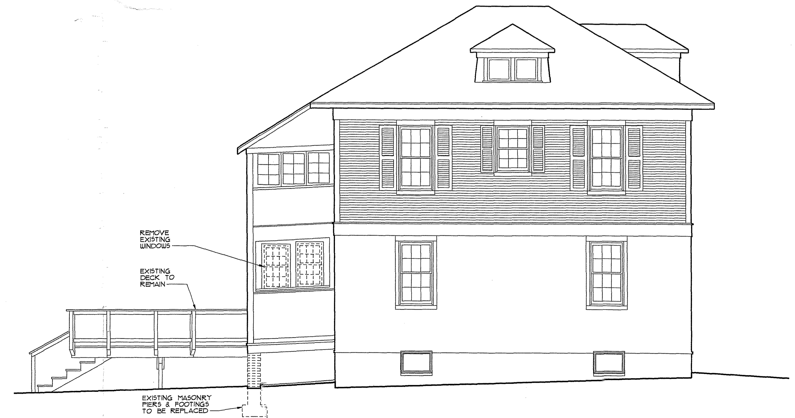
3 DEMOLITION NORTHWEST ELEVATION SCALE: 1/4" = 1'-0"
