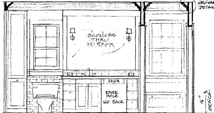
BB- TOILET, VANITY & BENCH WALL
