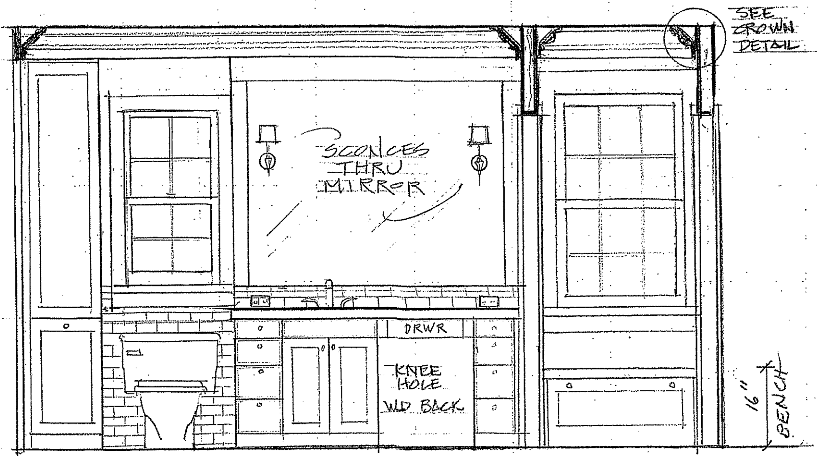
BB-TOILET, VANITY & BENCH WALL
