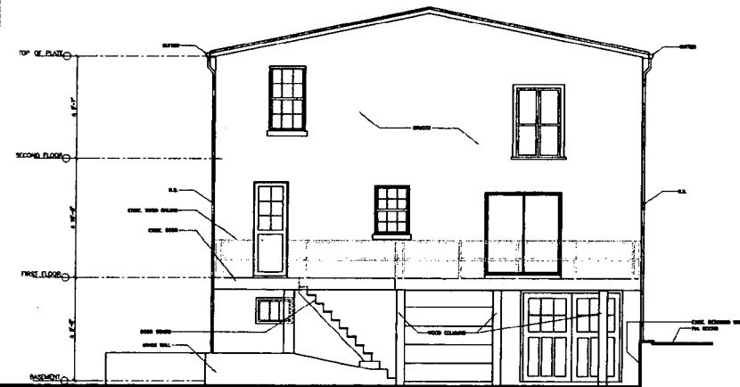
EXISTING REAR ELEVATION 1/4"=1'-0"
