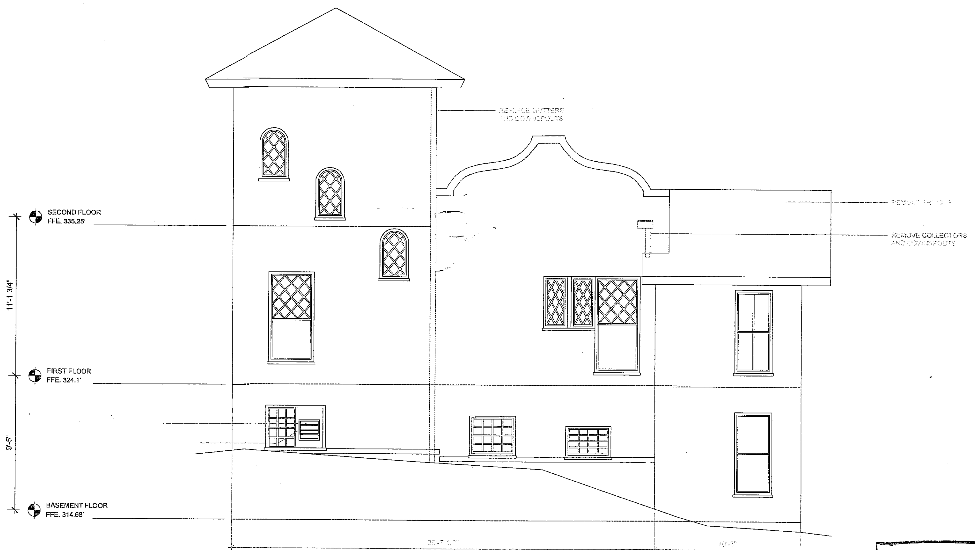
2 WEST DEMOLITION ELEVATION A5.2 SCALE: 1/4" = 1'-0"
