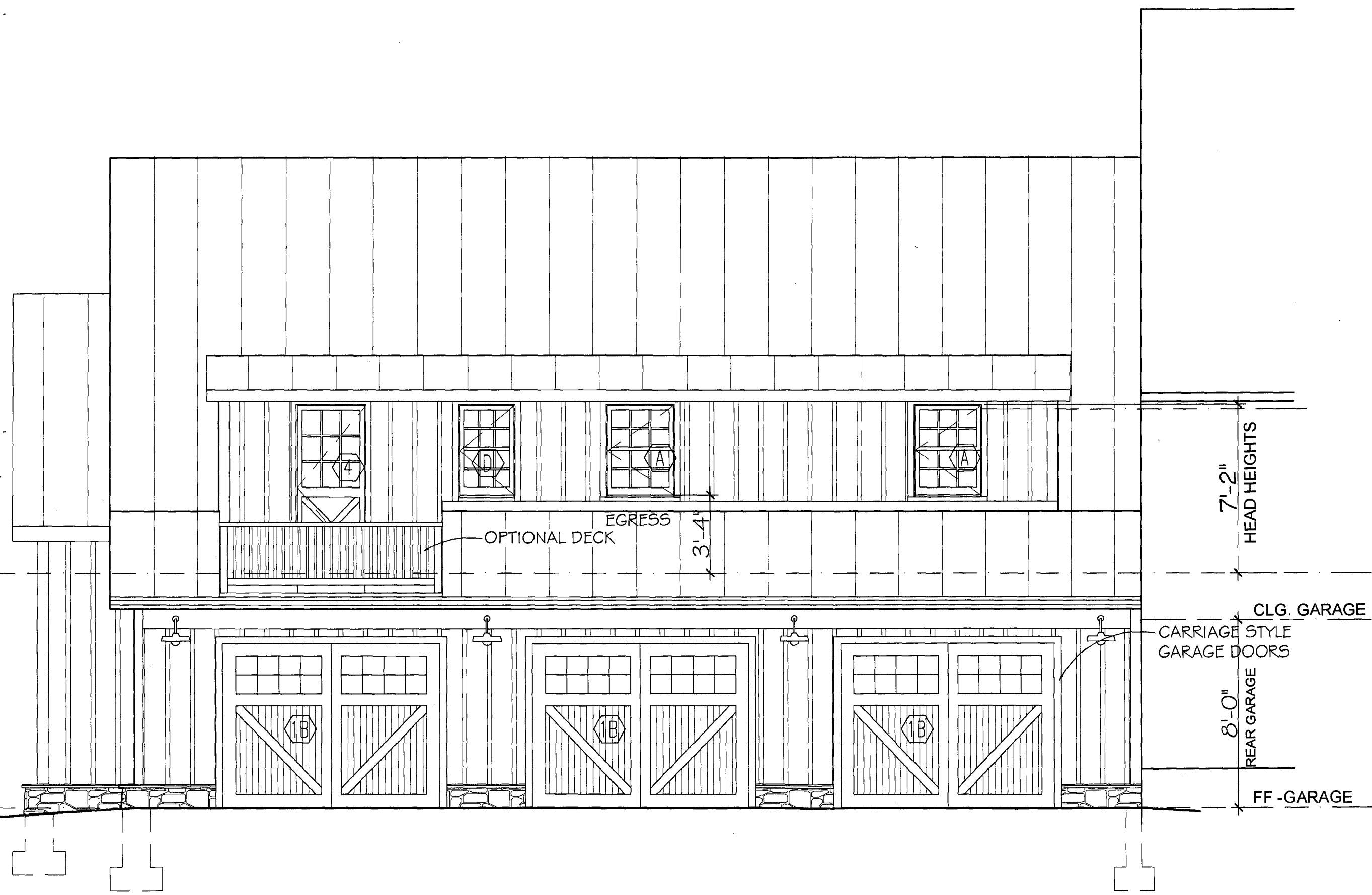
1 GARAGE REAR ELEVATION 1/4" = 1'-0"
