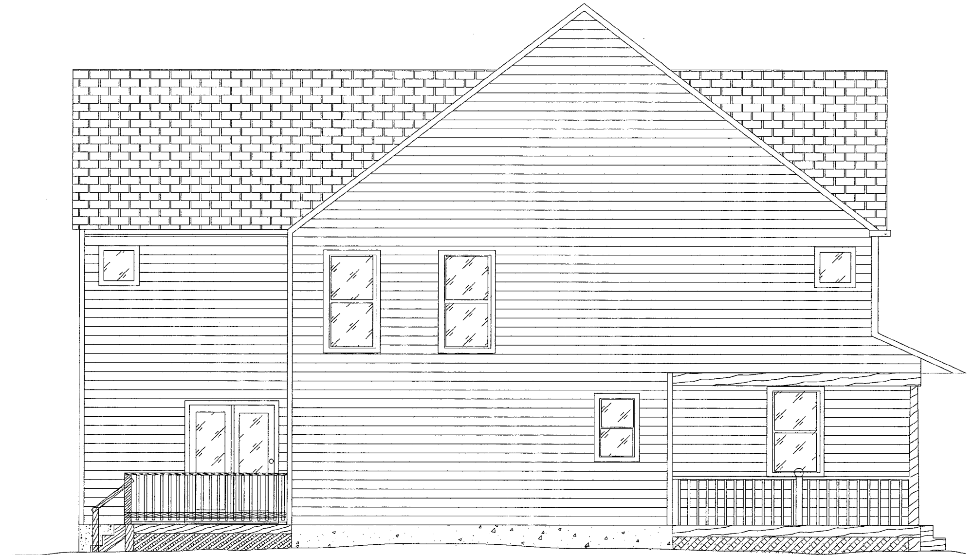
10005 Leafy Avenue North Side Elevation (current) with wood deck in 12X12 notch in foundation at northeast corner Scale 1:62.5
