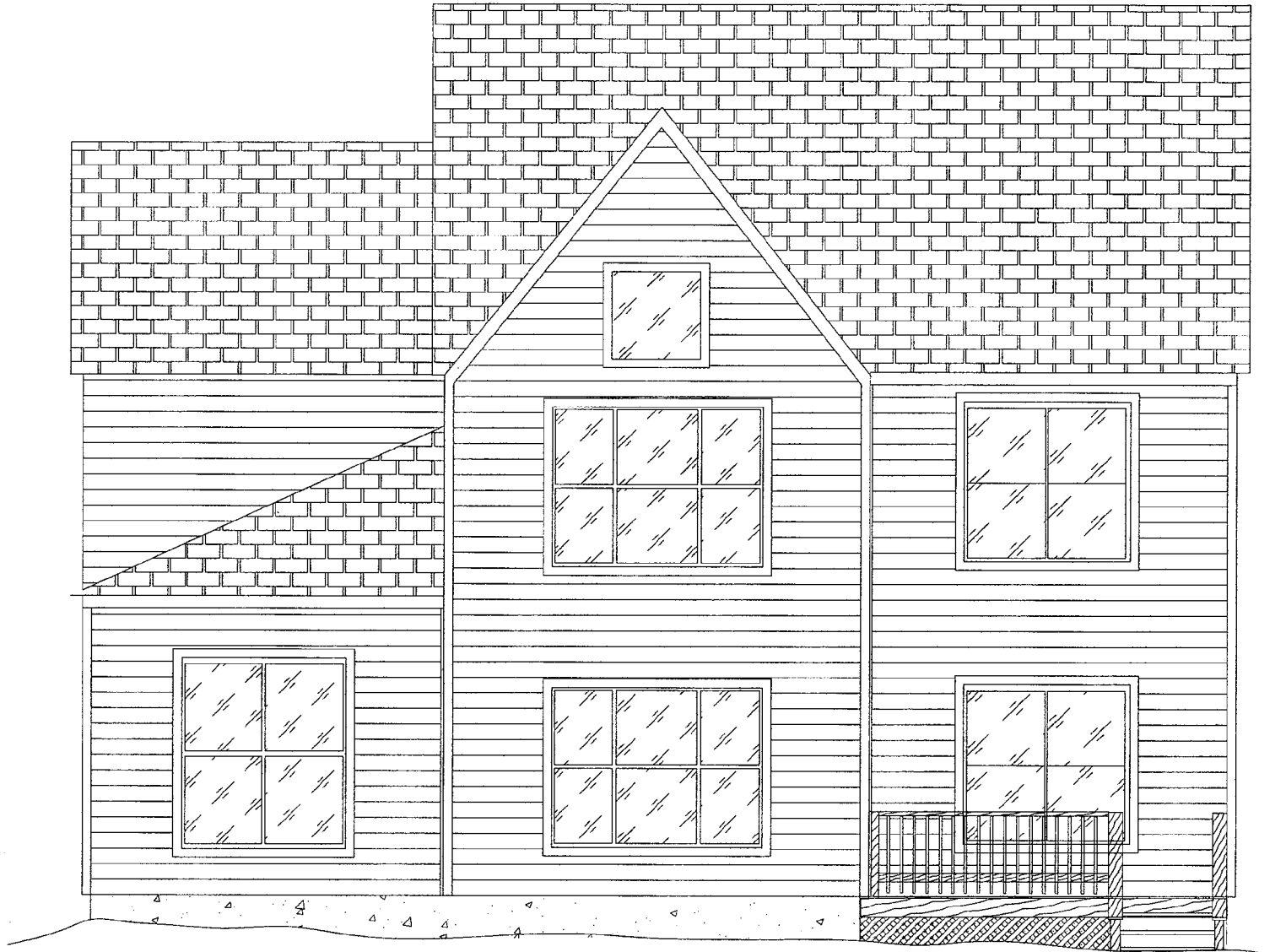
10005 Leafy Avenue East Side Elevation (current) with wood deck in 12X12 notch in foundation at northeast corner Scale 1:62.5
