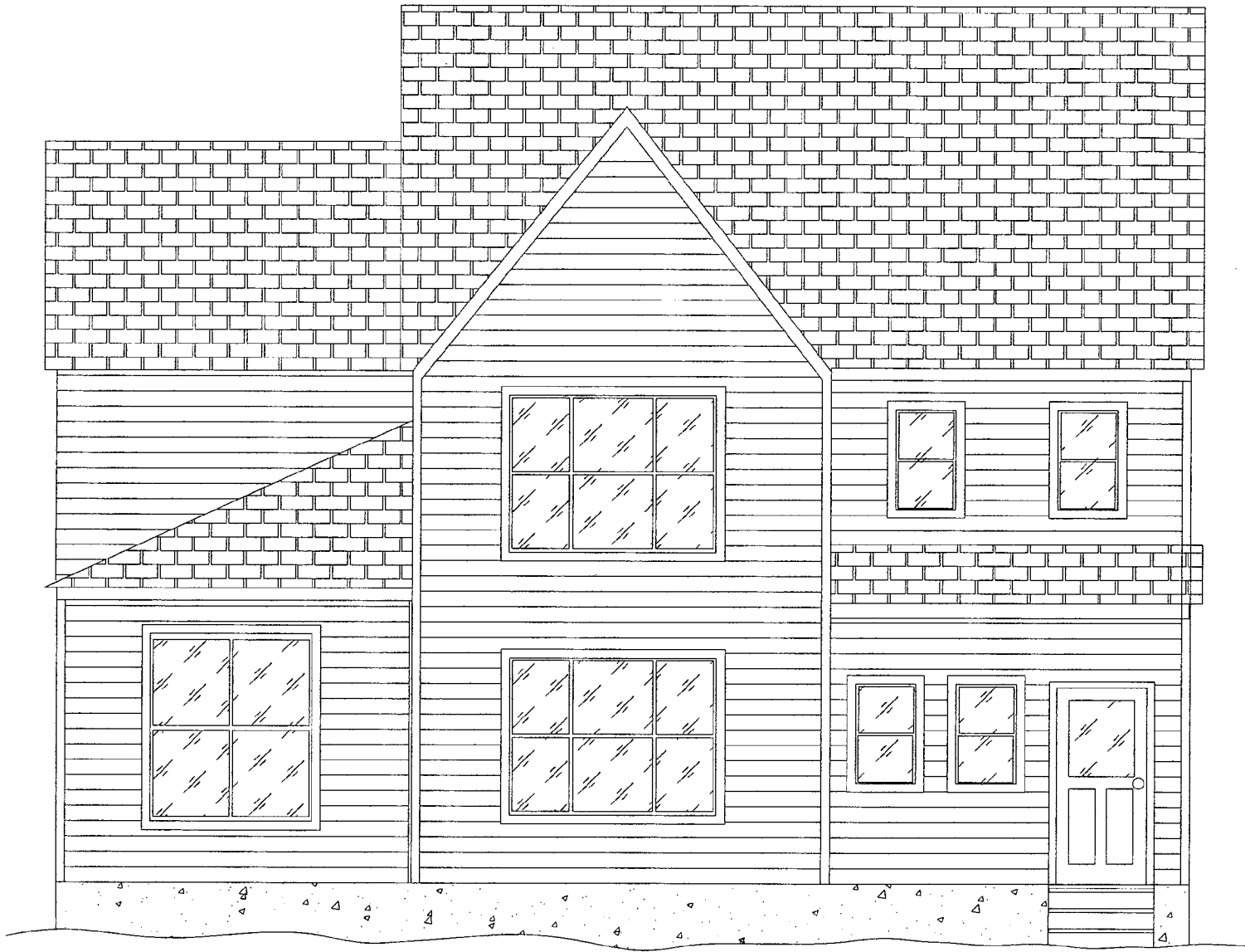
10005 Leafy Avenue East Side Elevation (proposed) with sunroom addition in place of deck at 12x12 notch in foundation at northeast corner Scale 1:62.5
