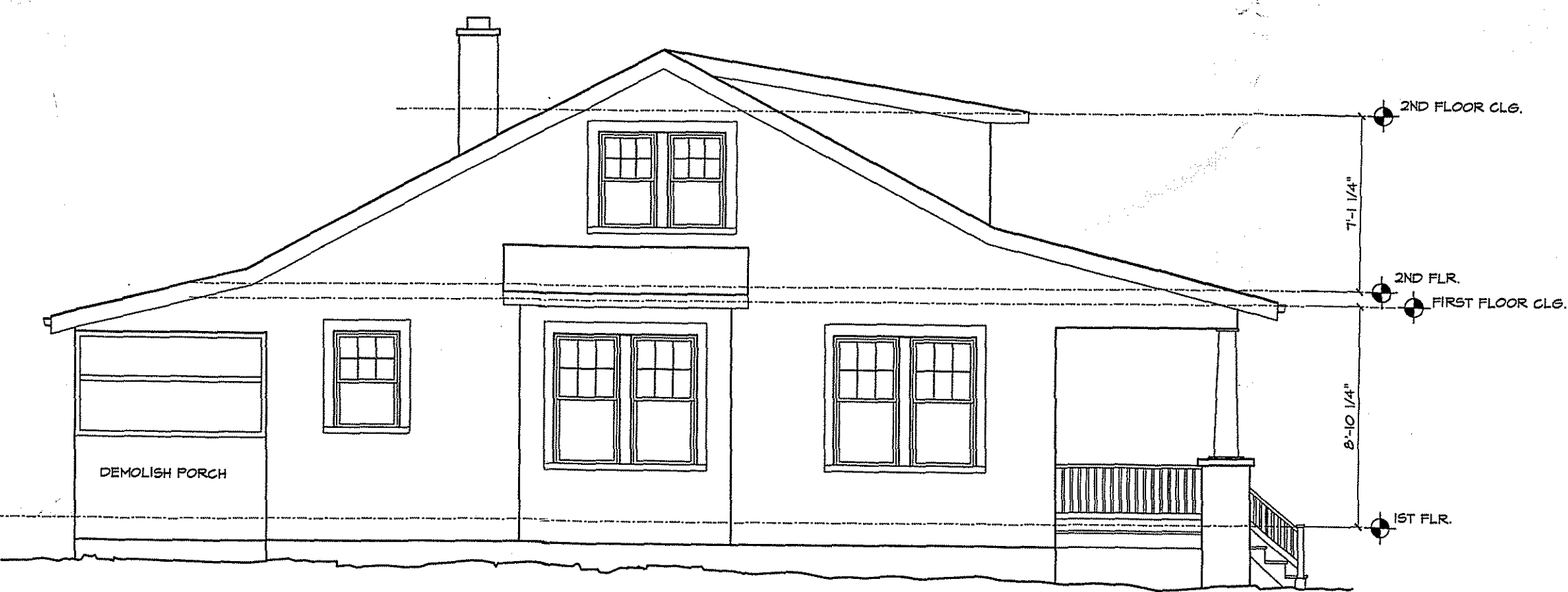
EXISTING LEFT ELEVATION 3/16"=1'-0"
