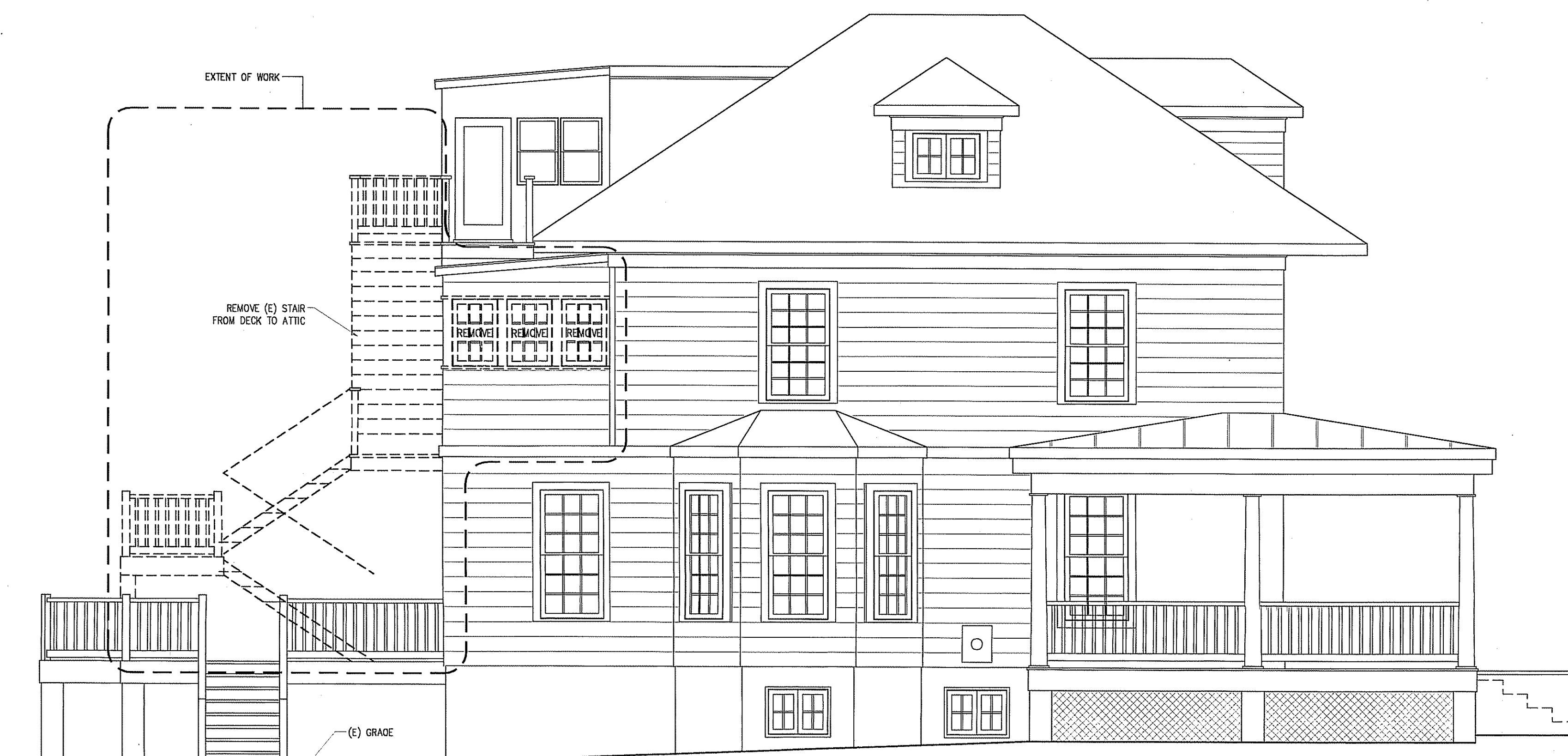
EXISTING/DEMOLITION 4 WEST ELEVATION D102 | SCALE: 1/4"=1'-0"
