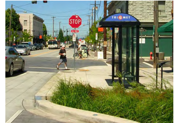
Figure 42: Example of a bus bulb located near an intersection to provide direct access for people utilizing public transit.
