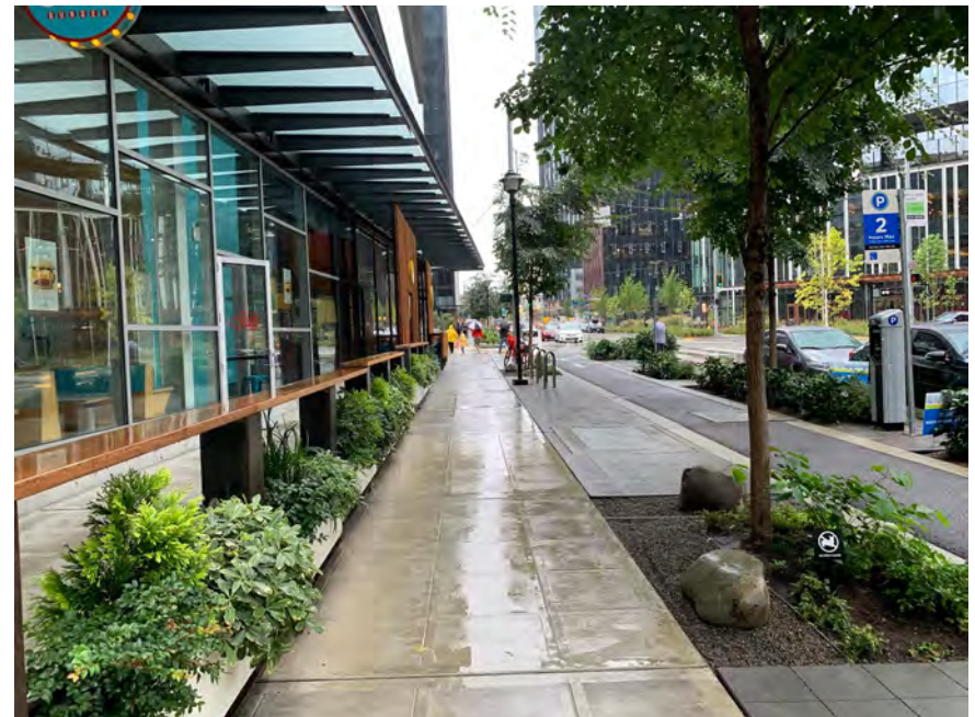
Figure 35: Landscaping and seating provides definition between sidewalks and separated bike lanes.
