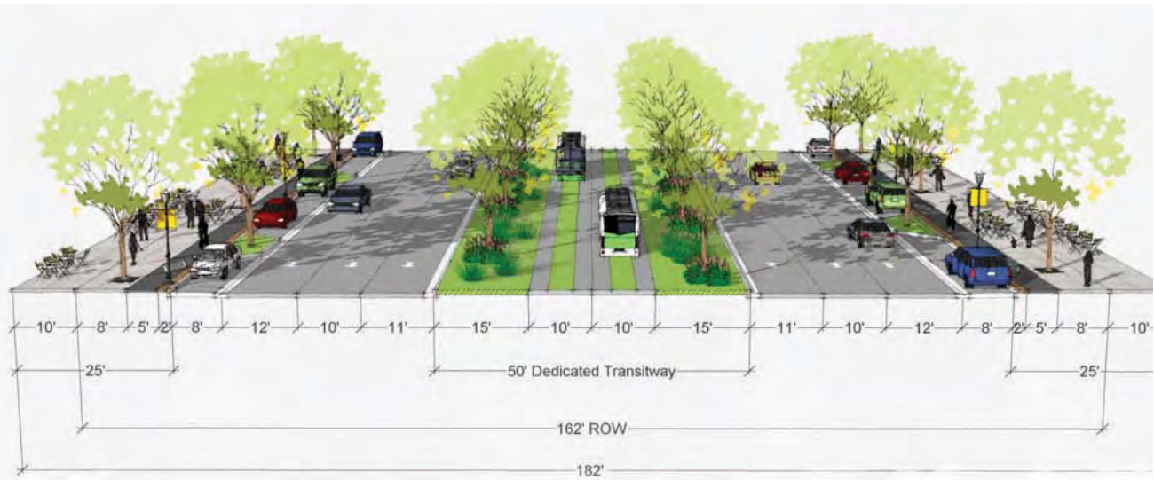
Figure 88: An alternative cross section for Rockville Pike including bus rapid transit in the median, as recommended in the Sector Plan.
