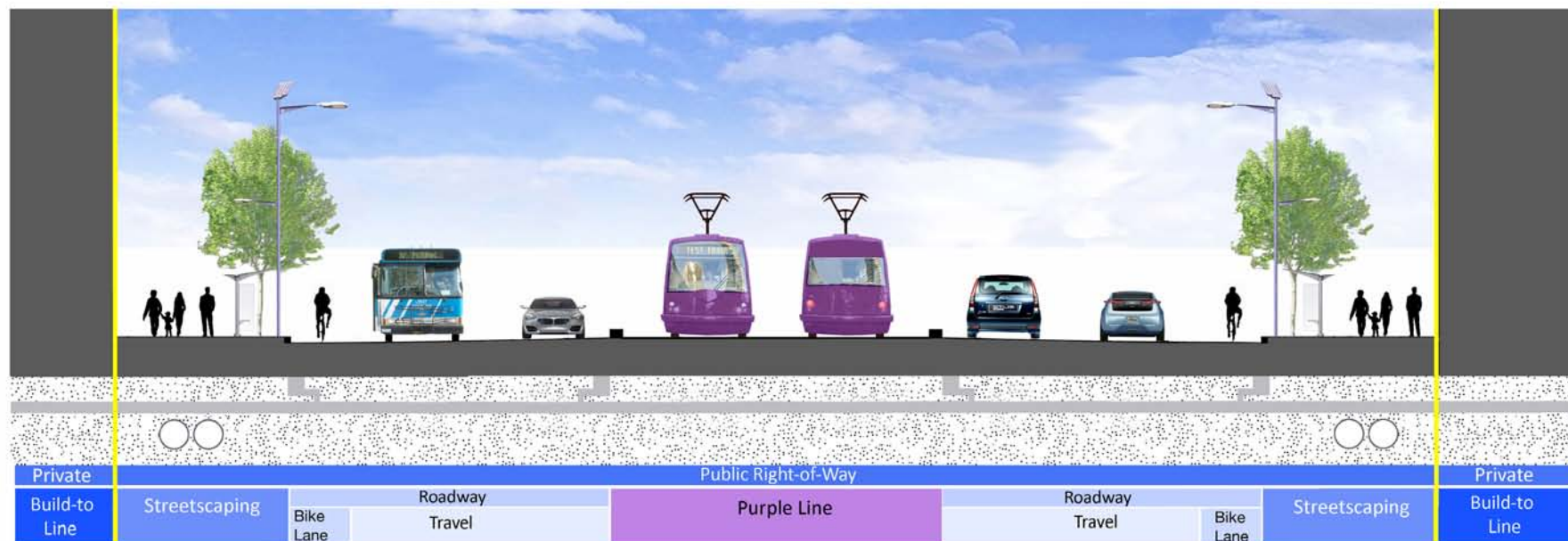
Illustration 11 Piney Branch Road Cross Section between Arliss Street and University Boulevard
