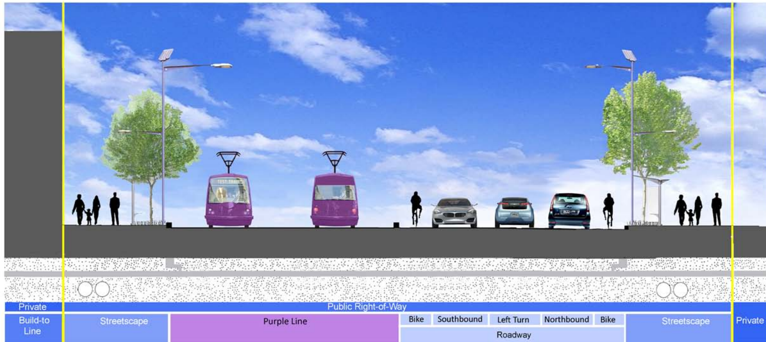
Illustration 7 Arliss Street Cross Section Street Level
