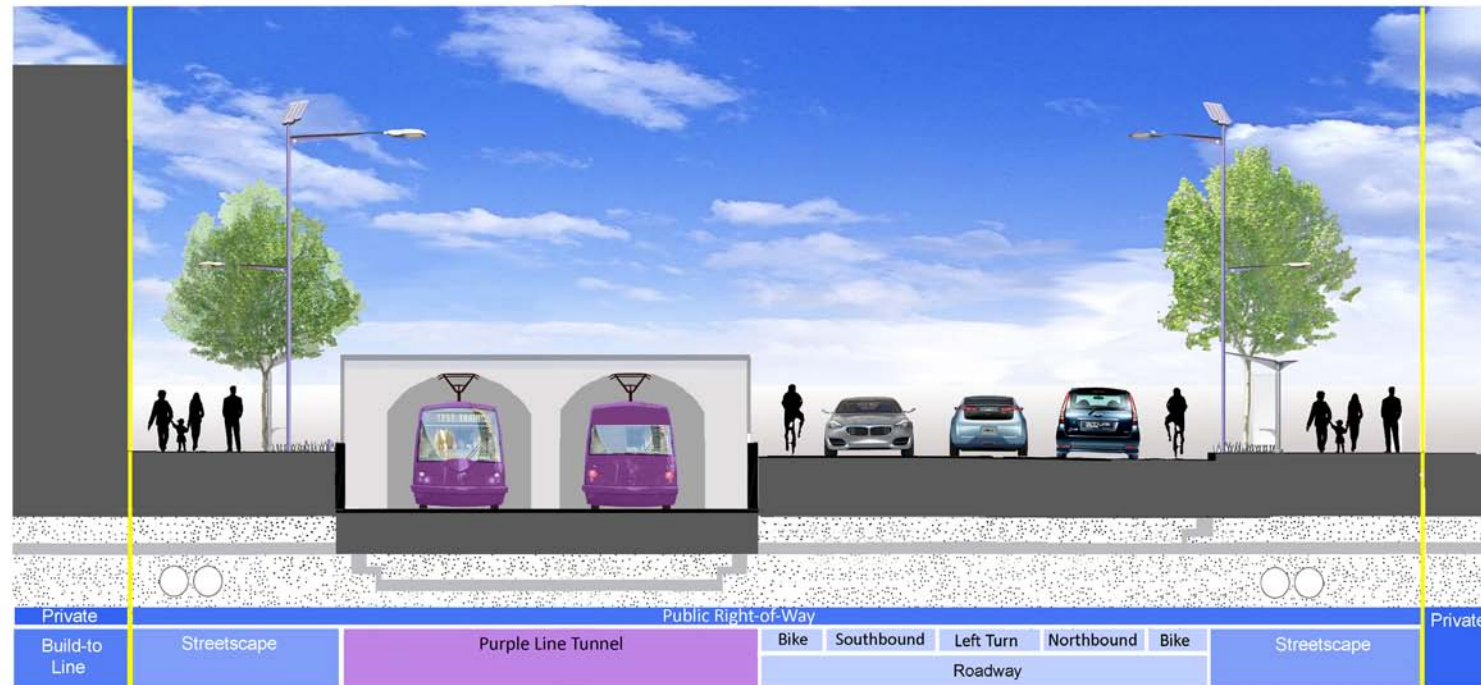
Illustration 6 Arliss Street Cross Section at Tunnel
