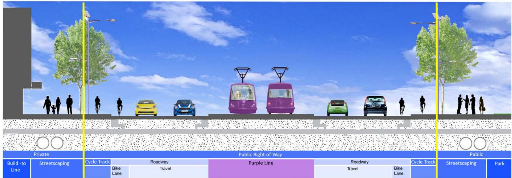
Illustration 18 University Boulevard Cross Section between Seek Lane and Bayfield Street
