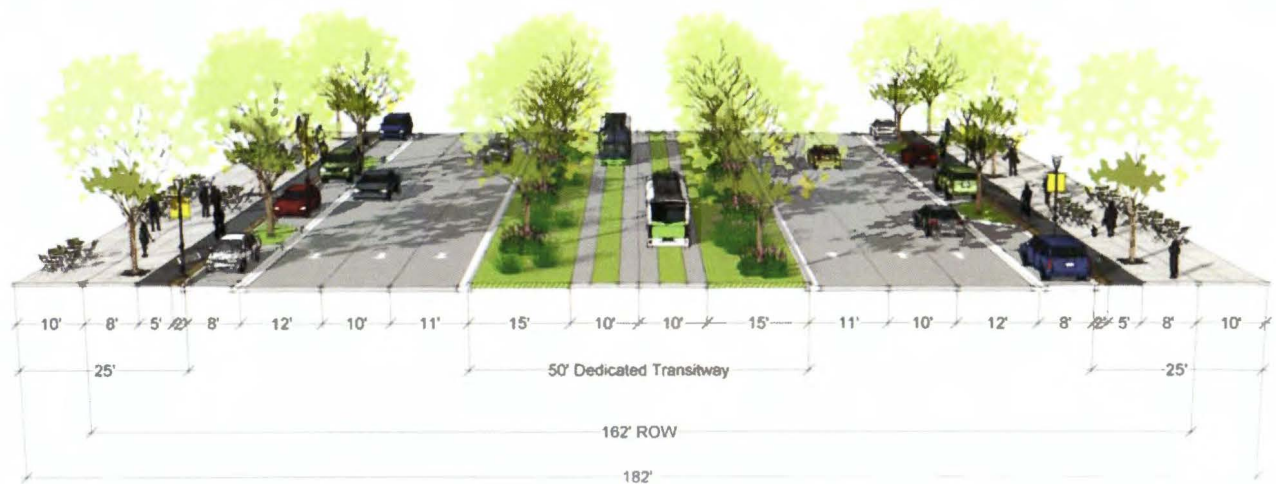
Figure 2: Alternative Rockville Pike BRT Cross Section
